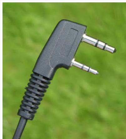
The connections are helpfully marked on the PCB, so all that was required was a continuity test to find which part of the jack plug was connected to which wire in the microphone. The unused (tip of the 3.5mm plug and ring of the 2.5mm plug) are presumably for the USB programming connection.
