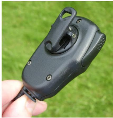
There is a useful clip on the back which partially obstructs the top screw, you need a well-fitting screwdriver to avoid slipping out of this.
