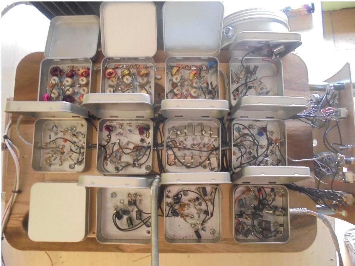
Exact copies for the HF amplifier, mixer and IF amplifier of the Bitx schematic.
