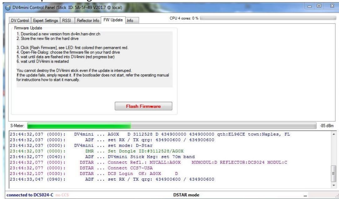
A file selection window opens and you select the new firmware file. This makes the LEDs on the DV4mini blink in different colors and when it is finished the blue light is on solid.
