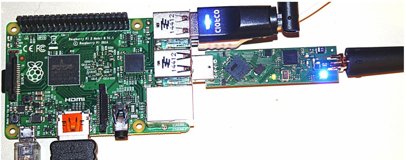
The dongle on the top is a WiFi stick to connect to the internet. Below you can see the DV4mini. The board also has connectors for a keyboard, a mouse and a HDMI display. This configuration allows for a low power operation.
