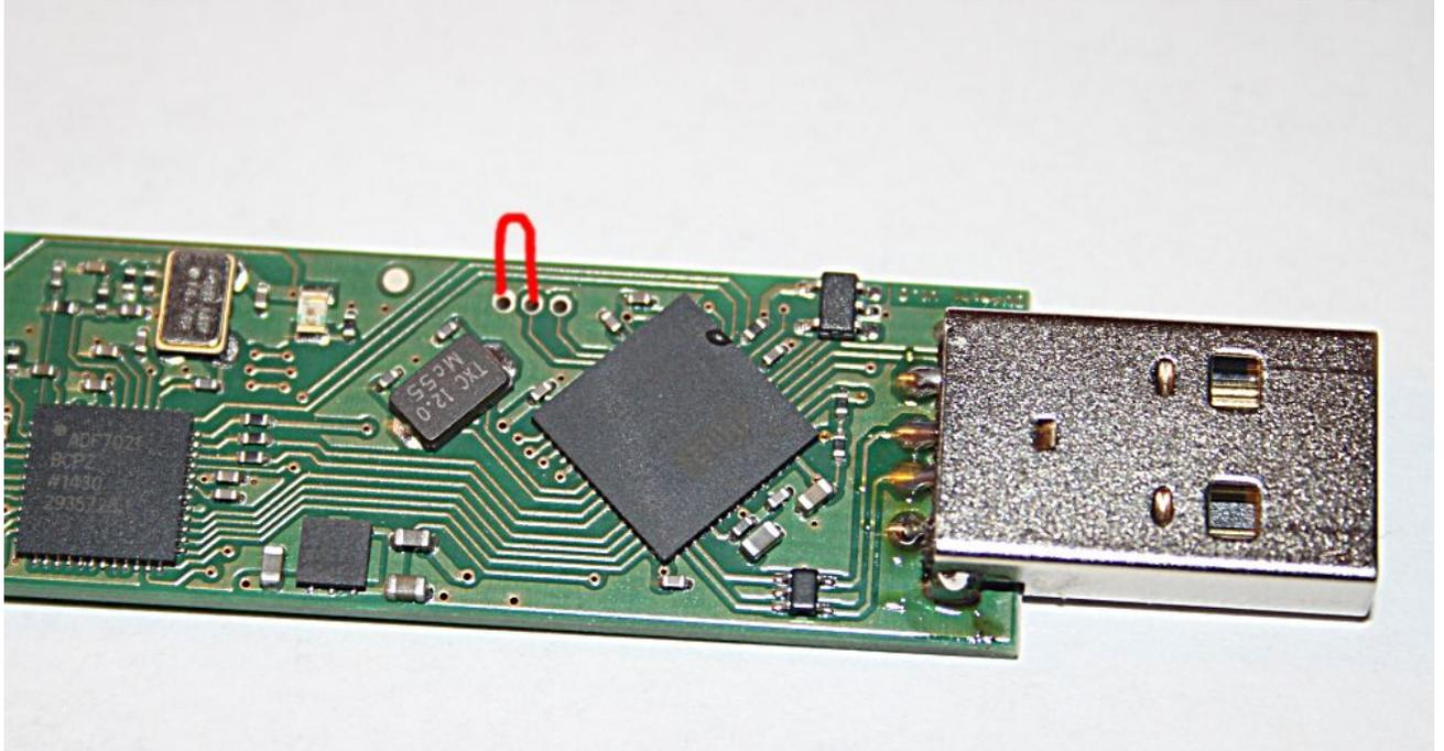
You need to connect the red marked points for example with tweezers **while** inserting the DV4mini into the USB interface. The boot loader will start with LEDs in color. Now you can start the user interface dv4mini. Go to expert settings load the new firmware by clicking on "Flash Firmware".
