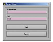
This window sets the address of the communication equipment. After the input of the IP address of the equipment, the setup is completed by clicking the Set button. The IP address of Spectrum Analyzer in the Internet should be entered correctly. The port number is set to 5000.
