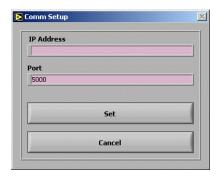
Upon the execution of the Ethernet Graphic User Interface program, the main window and IP address setup window are displayed at the same time as above. Then, the IP address of the equipment to be connected is entered. By clicking the Set button, IP address setup is completed. Note that the IP address of the Spectrum Analyzer which is connected to the Internet should be specified correctly. The port number is set to 5000.
