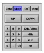
By using the Keypad input, Center frequency, Span frequency, Reference level and Step frequency can be set. Alternatively, the setup value can be modified by using the UP or DOWN button conveniently.
