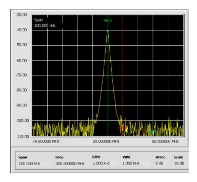
Below the graph display, current center frequency, span frequency, RBW, VBW, Atten, scale and frequency step are shown. On the upper right, LED is displayed to show the current communication state.
