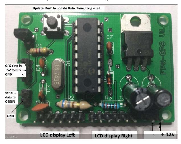
Connect the 2x16 LCD display with the supplied 6pin flatcables. On the GPS board left pin from LEFT connector to the left pin from LEFT connector on the LCD. And so on for all 12 wires. Straight cables.
