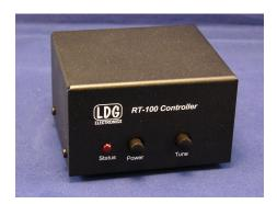
**Important Note:** The transmission line between the RC-100 and the RT-100 tuner must <u>never be grounded</u>. Doing so would cause the RC-100 to attempt to source 12 vdc directly to ground, damaging the unit. Never use coax switches that ground unselected ports even momentarily.
