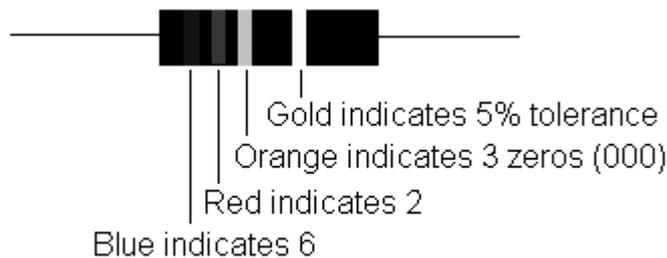
The value of this resistor is  $62000 \Omega$  or  $62 \text{ k}\Omega$
