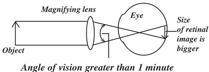
When we look at an object or a part of that object, the *angle of vision* should be wider than one *minute* (a unit of angular distance equal to a 60th of a degree) for the formation of an image of distinguishable shape. If the *angle of vision* is less than one minute, the image of an object appears to be just a '*point*' to our eyes. When we view an object, which is far away (or if the object is too small), the object is observed with an '*angle of vision*' less than one minute.
