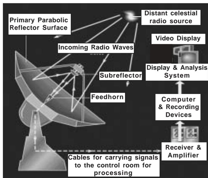
*Different stages of a basic radio telescope system*
