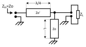
Impedance Matching with reactive compensation of the complex load
