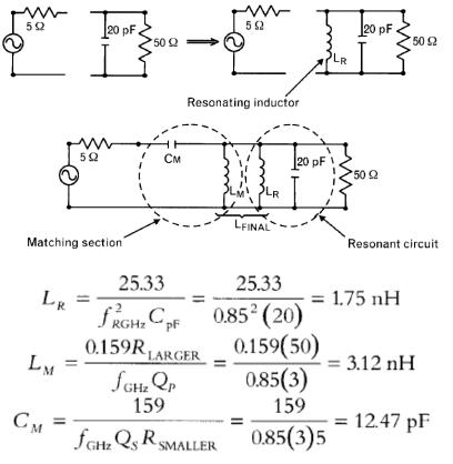
after that we can combine  $L_R$  and  $L_M$  in a single parallel inductor  $L_{MR}$
