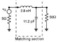
The unbalanced L-C circuit used to match 5  $\Omega$  to 50  $\Omega$  is a standard L-type matching network using a series L and a shunt C.
