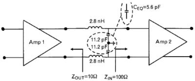
• After establishing the unbalanced matching circuits, the virtual ground can be eliminated. The two 11.2pF capacitors can be combined into a single floating 5.6pF capacitor. The two balanced ports are now matched to each other at desired frequency.
