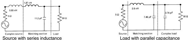
When the Q of a termination exceeds the limit set by the nodal-Q calculations, we need to neutralize the excessive amount of parasitic reactance.
