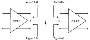
With the help of a virtual ground the balanced ports can be split into unbalanced ports. Input and output impedances of the unbalanced ports are half of the balanced ports.
