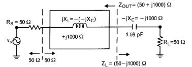
When  $R_s = R_L$  matching requires only a series reactive element
