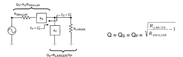
**3)** Knowing the Q-values, we can find the series and parallel elements, reactances, and get the values of the inductor and capacitor of the network using the following equations:
