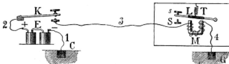
DIAGRAM ILLUSTRATING THE PRINCIPLE OF THE MODERN TELEGRAPH.
