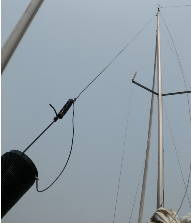
Sailboat Antenna and Loading Coil
