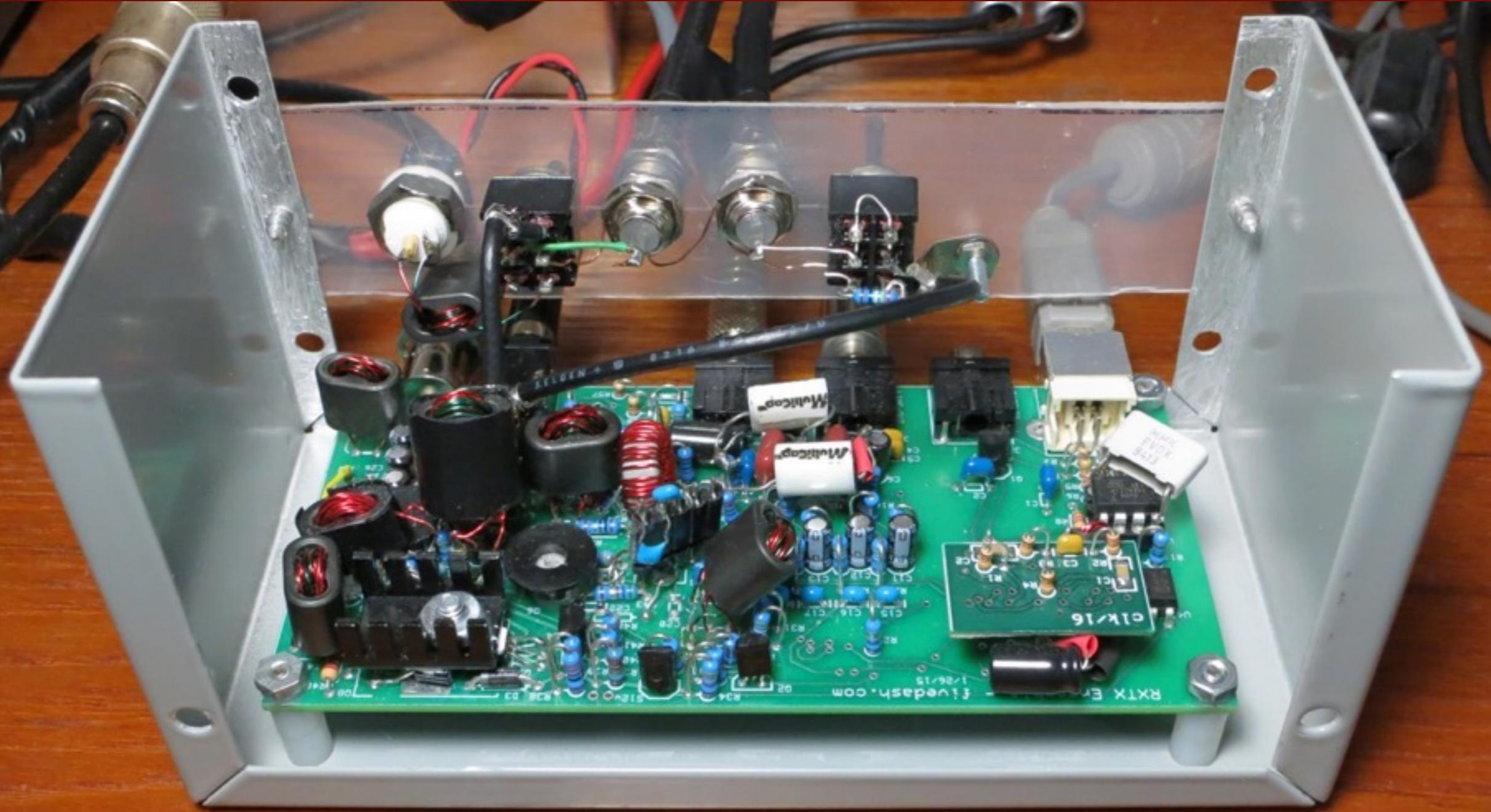
**Modified SoftRock RXTX Transceiver
