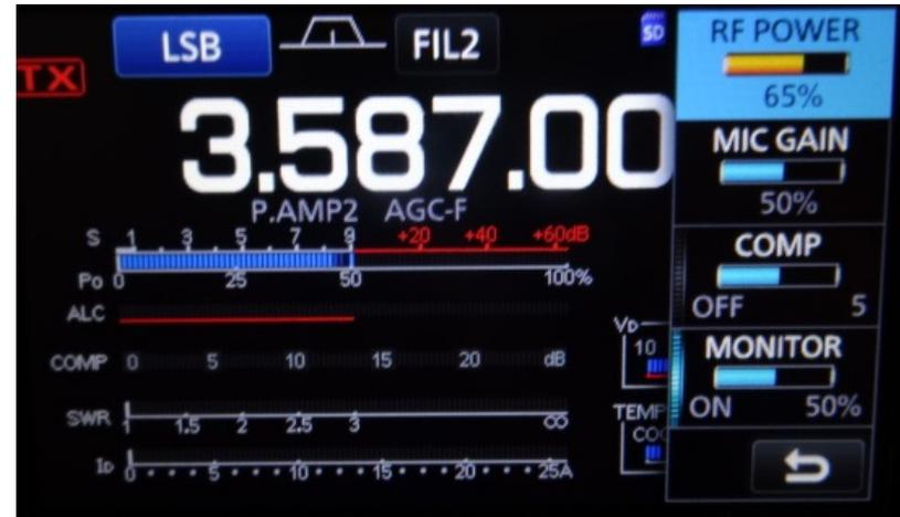
Image on left shows the 7300 screen in USB Data mode, notice no COMP section. Image on right shows the 7300 in LSB mode, notice the Multi Function includes COMP.
