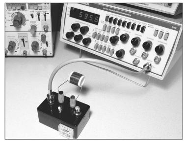
Figure 25.78 — The signal generator's output is 596 kHz (0.596 MHz) with the switch in the position selecting the 0.01 µF capacitor. Using the formula given results in an calculated inductance of 7.1 µH.
