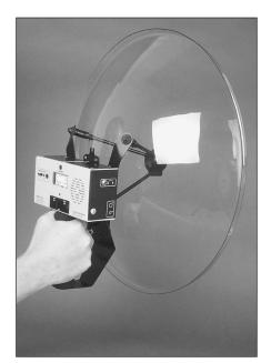
Figure 27.10 — The clear plastic parabolic dish is an "ear" connected to an ultrasonic detector that lets utility personnel listen for the sound of arcs.
