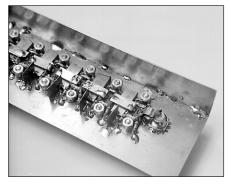
Figure 25.87 — The attenuator before final mechanical assembly. The 1/4-inch strips are spaced 0.033 inch apart to form a 50- $\Omega$  connection from the BNC connector to the stripline. There are 1/2-inch square shields between 10-dB sections. The square shields have a notch in one corner to accommodate the end of the rectangular tubing.
