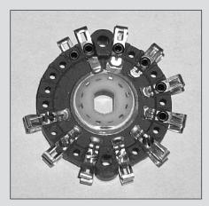
Figure 26.A1 — Five contacts starting at the 4:30 position on the wafer have been replaced using contacts removed from another switch and #2-56 hardware. [Photo courtesy of Matt Kastigar, N9ES]
