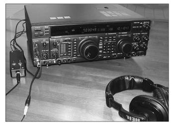
Figure 62 — The AIE takes up little desk space. It plugs inline between the transceiver and headphones and requires 13.6 V dc. In the author's shack, the unit is powered from a transceiver accessory jack and is always switched on.
