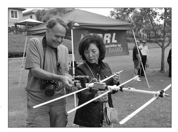
Figure 1.26 — **Amateur Radio Direction Finding** (ARDF) equipment need not be expensive. Yagis made from measuring tapes and PVC pipe are very popular for direction finding on 2 meters with a handheld transceiver. Here, Dan Slater, AG6HF (left), tests an antenna he built. [Joe Moell, KØOV, photol
