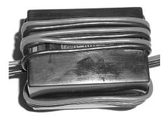
Figure 21.70 — RF choke for screwdriver antenna control and power leads.
