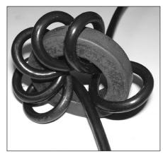
Figure 27.20 — To eliminate HF and VHF signals on the outside of a coaxial cable, use an 1- to 2-inch OD toroid core and wind as many turns of the cable on the core as practical.
