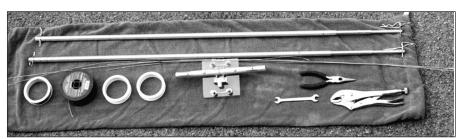
Figure 21.24 — The entire inverted-U antenna parts collection in semi-nested form, with its carrying bag. The tools stored with the antenna include a wrench to tighten the U-bolts for the mast-to-plate mount and a pair of pliers to help remove end wires from the tubing.
