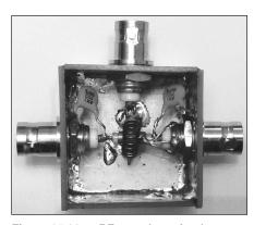
Figure 25.90 — RF sampler using box construction.
