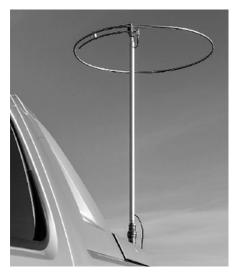
Figure 21.79 — The halo is a popular horizontally polarized mobile antenna for 6 meters through 70 cm. This version was made by Jerry Clement, VE6AB, and the construction article is available online (see text).
