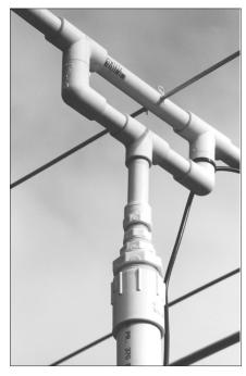
Figure 21.90 — The completed 2 meter Yagi is shown with the PVC boom and mast mount.
