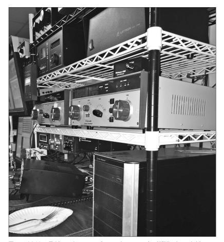
Figure 24.16 — Taking advantage of a good opportunity, NØNI adapted this set of metal wire shelving to hold his equipment. The wire shelves also act as an RF ground plane and provide ventilation. [Bob Lee, WØGXA, photo]
