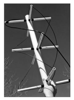
Figure 56 — This view shows the QHA with all four legs in place. The ends of the PVC cross arms that hold the coaxial leg are notched; the wire elements pass through holes drilled in the ends of their supporting cross arms.
