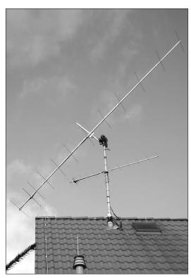
Figure 66 — The 12-element Yagi used by DL1VPL to complete DXCC on 144 MHz.
