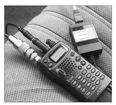
Figure 6 — A 2-meter FM handheld transceiver attached to an APRS position encoder.
