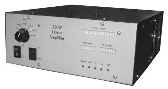
Figure 17.45 — This 250 W amplifier for 160 through 6 meters provides a detailed design example as well as a practical project. Additional photos and information about the interior layout may be found with this book's downloadable supplemental content.
