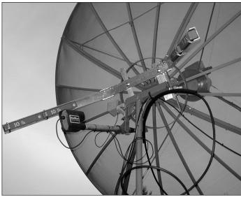
Figure 74 — Mounting arrangement, counterweights and az/el control system for the VA7MM 3 m dish.
