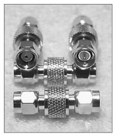
Figure 13 — RP connector adapters.
