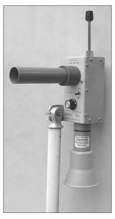
Figure 27.11 — The Radar Engineers Model 247 Hotstick Line Sniffer is an RF and ultrasonic locator. It is used by utility workers to pinpoint the exact piece of hardware causing a noise problem. Mounted on a hotstick, the sniffer is used from the ground or from a bucket.
