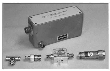
Figure 25.40 — Various RF test accessories. At the rear is a 10 dB step attenuator with a 0-120 dB range. In the foreground from left to right are a BNC "T" connector, a  $50-\Omega$  feed-through termination, a 0.1-500 MHz low-noise amplifier, and a 10-dB fixed attenuator.
