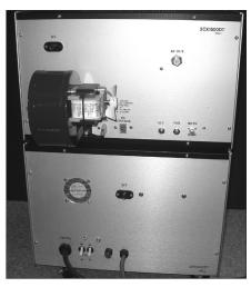
Figure 17.56 — At the top, front panel view of RF Deck and Power Supply for 3CX1500D7 amplifier. At bottom, rear view of RF Deck and Power Supply.
