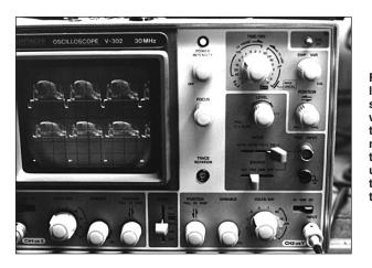
Figure 13 — An oscilloscope used to observe a video waveform. The lower trace is the video signal as it comes out of the sync stretcher. The upper trace is the detected RF signal from the amplifier.
