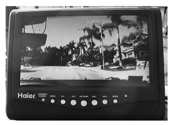
Figure 18 — Mobile ATV as shown here with a portable TV works fine using D-CATV 64-QAM, but it exhibits occasional freeze or tile effect from drop outs and multipath.
