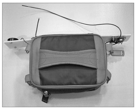
Figure 16.13 — The complete Near Space Tracker assembled in an insulated fabric lunch cooler.
