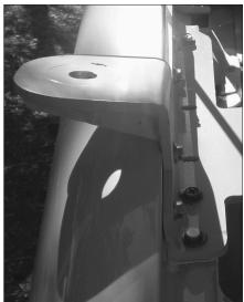
Figure 21.76 — The KE5DKM bracket mounts under the hood of a motor home.
