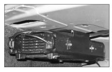
Figure 24.25 — The main body of the radio may be mounted in the vehicle's trunk or other out-of-the-way spot. Allow for plenty of ventilation.
