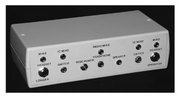
Figure 65 — Rear view of the audio interface box. Operator jacks are on the right, logger on the left. Connections to the radio are in the center.
