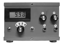
Figure 7.55 — The front panel of the fouroutput switching supply.
