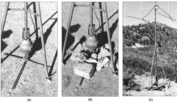
Figure 24.35 — The portable mast and tripod by WA7LYI. At A, the tripod is clamped to stakes driven into the ground. The rotator is attached to a homemade pipe mount. At B, rocks piled on the rotator must keep the rotator from twisting and add weight to stabilize the mast. At C, a 10 foot mast is inserted into the tripod/rotator base assembly. Four 432 MHz Quagis are mounted at the top.
