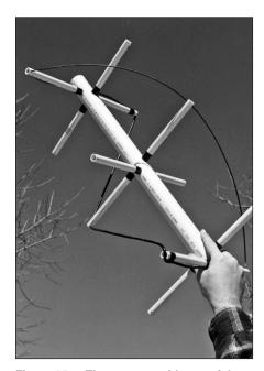
Figure 55 — The antenna with two of the four legs (filars) of one loop attached.
