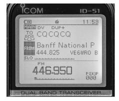
Figure 21 — The Icom ID-51A is a 2 meter/70-cm handheld with D-STAR functionality.
