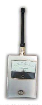
Figure 25.57 — The VE7NI field-strength meter.
