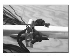
Figure 21.43 — Guys are made of Dacron line that is attached to the HVD by a stainless-steel worm-screw-type hose clamp. A self-tapping sheet-metal screw (not visible in the photo) prevents the clamp from sliding down the antenna.
