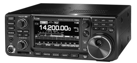
Figure 11 — The Icom IC-7300 is a a full-SDR (direct-sampling) transceiver in a conventional HF transceiver package. Instead of the more conventional up- or down-converting architecture, digitization is performed directly at the RF signal frequency.
