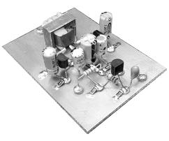
Figure 23.7E — The completed homebrew Audio Amp assembly shows simple, effective use of SMT components used together with conventional leaded components when constructed "Manhattan-style."
