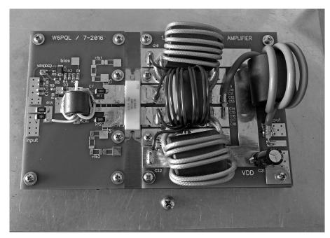
Figure 17.44 — Typical HF amplifier "pallet" designed by Jim Klitzing, W6PQL (www. w6pql.com/index.htm). This design is capable of 1 kW output power and uses the NXP BLF188XR LDMOS amplifier transistor module. [Jim Klitzing, W6PQL, photo]
