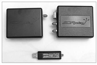
Figure 41 — Some examples of software defined receivers used for satellite operating. Upper left: SDRplay RSP1. Upper right: SDRplay RSP2. Bottom center: FUNcube Dongle Pro+.
