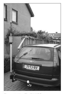
Figure 21.74 — The PA3VOS antenna mount easily supports a large screw-driver antenna and is offset to allow the hatch to open and close without removing the antenna.
