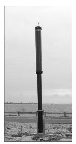
Figure 21.69 — The screwdriver-style remotely-controlled whip antenna. A small motor in the base mast moves a coil past contacts at the top of the metal base section. The top whip section is attached to the top of the coil. As the coil moves out of the mast, more inductance is connected in series between the base section and top section. Screwdriver antennas are popular because they offer multiband coverage. [Joel Hallas, W1ZR, photo]
