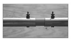
Figure 21.41 — The center insulator of the 15 meter HVD is a 1 foot length of 0.75 inch fiberglass rod. Insulator and elements have been drilled to accept #8 hardware.
