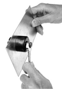
Figure 23.3 — A socket punch is used to punch a clean, round hole in sheet metal.
