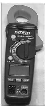
Figure 26.2 — A clamp-on meter probe is used with a digital multimeter for measuring ac current (left). Meters are also available integrated with the clamp-on probe (right).
