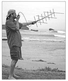
Figure 1.18 — Sean Kutzko, KX9X, uses a handheld antenna to make contacts through an Amateur Radio satellite. [Ward Silver, NØAX, photo]
