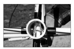
Figure 58 — An end-on view of the top of the QHA prior to soldering the loops and installing the PVC cap.
