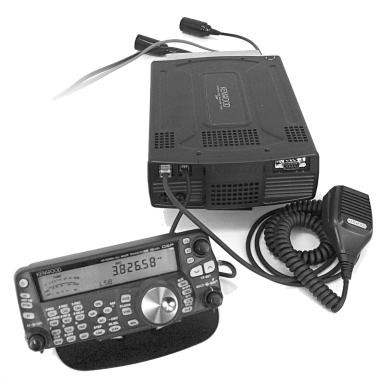
Figure 8 — Kenwood TS-480HX, the only transceiver in this category with a 200 W transmitter. The TS-480SAT looks similar, but offers 100 W output and an internal antenna tuner.
