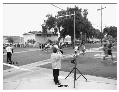
Figure 24 — A low power 50 mW battery operated portable 70 cm AM ATV transmitter is ideal for short range line of sight paths of up to 2 miles using 5 element beams. This setup can be used to show a critical intersection or condition of runners as an early warning to emergency response and aid station volunteers at races.
