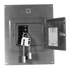
Figure 28.2 — If the switch box feeding power to your shack is equipped with a lock-out hole, use it. With a lock through the hole on the box, the power cannot be accidentally turned back on. [Photo courtesy of American ED-CO]
