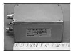
Figure 35 — This downconverter by Downeast Microwave converts signals at 2.4 GHz to 2 m. With its weatherproof enclosure, it is designed to be installed at the antenna.
