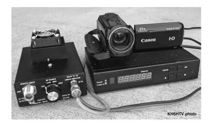
Figure 4 — The Hi-Des HV-100EH DVB-T modulator is shown here driving a KH6HTV 70-7B linear amplifier on the 70 cm band. The modulator also tunes the 33 cm band and has an adjustable output up to -3 dBm for driving a high linearity MMIC and FET power amplifier. Transverters can be used for operation on the higher frequency bands.
