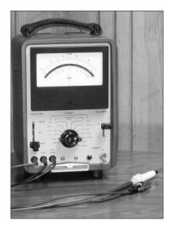
Figure 25.3 — This classic Hewlett-Packard HP412A vacuum-tube voltmeter (VTVM) has specifications that put many modern solid-state multimeters to shame.
