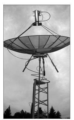
Figure 73 — This 3 m TVRO dish with aluminum frame and mesh surface was outfitted for 1296 MHz EME as a joint effort by VA7MM and VE7CNF. The dual-circular polarization feed is a VE4MA/W2IMU design.
