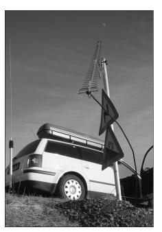
Figure 67 — TF/DL3OCH used a rural road sign to help him give contacts with Iceland to a number of EME operators on 1296 MHz. Bodo has activated many DXCC entities on 1296 MHz EME by using JT65, a single long Yagi and a 100 W solid state amplifier.
