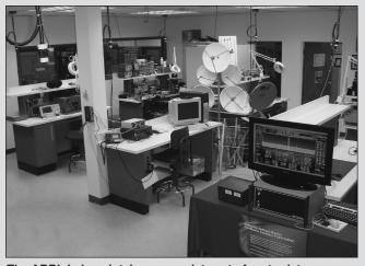
The ARRL Lab maintains a complete set of up-to-date equipment as well as an RF-tight screen room for Product Review testing. [Bob Allison, WB1GCM, photo]
