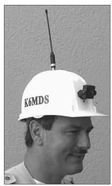
Figure 33 — Michael Saculla, K6MDS, built an ATV Hat Cam — www.hamtv.com/hatcam.html — using a CMOS color camera along with a Videolynx 70 cm transmitter for public service applications.
