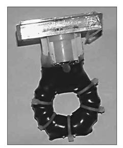
Figure 25.83 — Assembly of the RF current probe. Use an all-plastic meter and mount the circuits and toroid directly on the back of the meter case.
