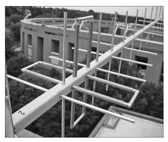
Figure 72 — Dual-polarization EME array at W2PU. At the left, shows the four 15-element, rear-mounted Yagis. Boom length is 3.5 m, and stacking distance is 1.2 m in each direction. The right photo is a close-up showing some details around the driven loops.
