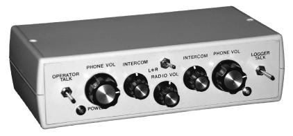
Figure 63 — Front view of the audio interface box. Operator controls are on the left and logger controls are on the right.
