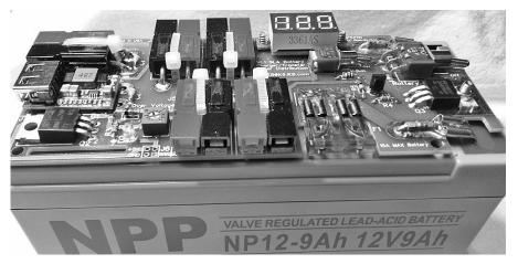
Figure 7.67 — The charging circuit shown mounted directly on a 9 Ah SLA battery. Note the USB charging module mounted next to J1 at the left-hand side of the board.
