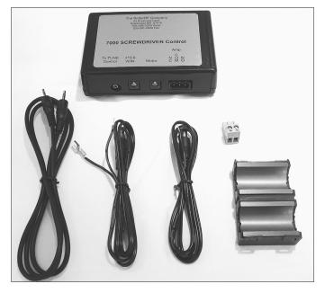
Figure 21.73 — A screwdriver antenna controller made to work with the IC-7000 transceiver.
