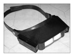
Figure 23.6 — A magnifying visor is great for close-up work on a circuit board. These headsets are often available for less than \$10 at hamfests and some even come with superbright LEDs mounted on the side to illuminate the components being soldered.
