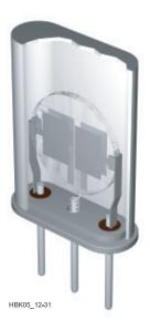
Figure 10.46 — A dual monolithic crystal filter has two sets of electrodes acoustically coupled to provide a two-pole response in a single crystal unit. The center lead is connected to the case and grounded in normal operation.
