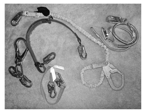
Figure 28.20 —Left-to-right, a collection of locking clips, a belt-type positioning lanyard, a fall-arrest lanyard, and a versatile adjustable lanyard. [Don Daso, K4ZA, photos]
