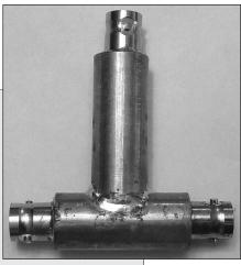
Figure 25.91— RF sampler using tube construction.
