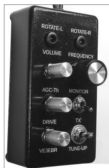
Figure 56 — The SDR Knob Box replaces software controls such as click boxes and sliders with physical knobs and switches read by an Arduino microcontroller and then relays the appropriate commands to an SDR transceiver.
