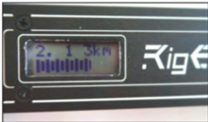
In a classic ARDF competition, the FoxRex 144 LCD display shows the frequency memory number, transmitter number, transmission time remaining, signal strength, and an estimate of distance to the transmitter. (Photo by Joe Moell, KØOV)
