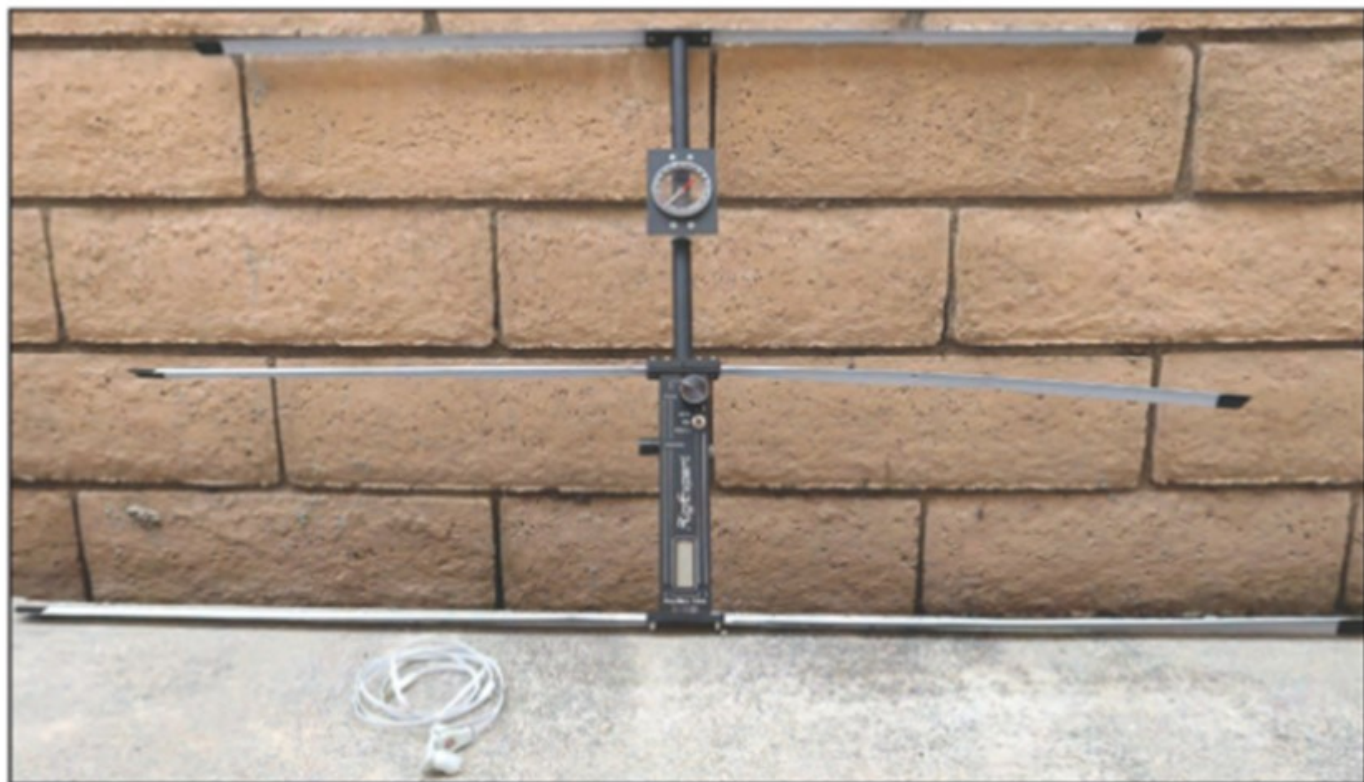
The new FoxRex 144 ARDF set has a measuring-tape Yagi for 2 meters and a sensitive AM receiver that is full of "bells and whistles." (Photo by Joe Moell, KØOV)
