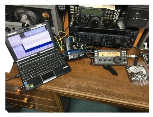
I used my Elecraft KX3 transceiver powered by the batteries that I normally use with my Ryobi power tools. As shown in the picture below, I cut off the handle of old drill and used it as a housing for the lithium ion drill battery. This makes for a rapid battery change and offers an easy way to connect the DC to Dc converter to the supply voltage. With the help and advice of Bob, K3DBD. I chose the adjustable QSKJ 1212CCBA-80W DC-
