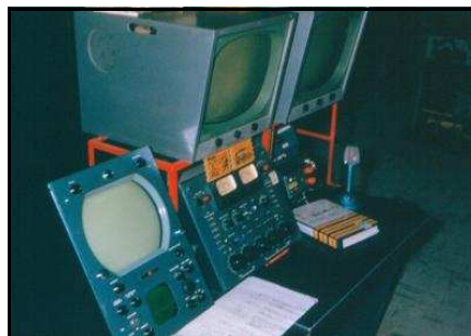
The Control console where video was switched between studio in Chocowinity and NBC. The two monitors up high monitored the NBC and studio feeds. Lower monitor was the transmitter input. Microphone was for 26 Mc (MHz) 2-way communications between transmitter and studio facilities. (Heard a lot of skip!) White paper on table was the program log that was followed by the engineer so he would know when station breaks came. No color monitor.
