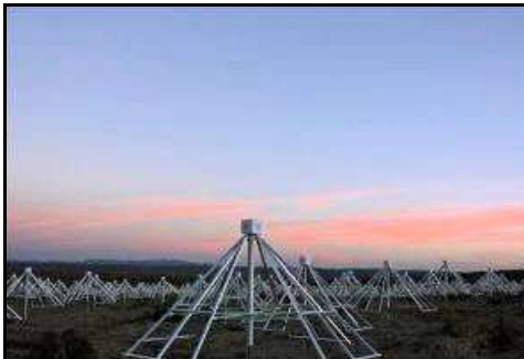
The Long Wavelength Array at Sevilleta National Wildlife Refuge is capable of imaging the entire sky at once, allowing AFRL scientists to track and characterize sporadic E. The facility consists of 256 dual-polarization dipoles. [Ken Obenberger photo]
