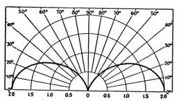
Fig. 2-36 — Vertical dipole antenna with center 1/4 wavelength high.
