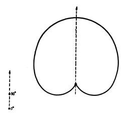
Fig. 4-25 — Representative pattern for a twoelement end-fire array with 90-degree phasing, in the plane perpendicular to the plane containing the elements.
