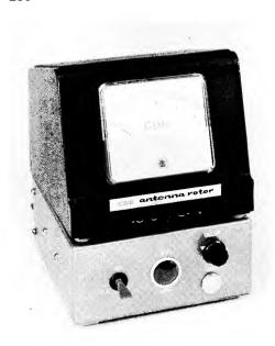
Fig. 14-2 — The Ham-M rotor control.
