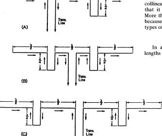
Fig. 4-12 — Three- and four-element collinear arrays. Alternative methods of feeding a three-element array are shown at A and B. These drawings also show the current distribution on the antenna elements and phasing stubs. A matched transmission line can be substituted for the tuned line by using a suitable matching section.
