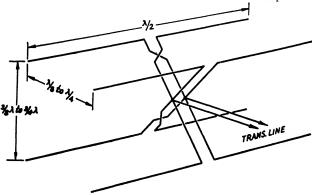
Fig. 16-8 — Four-element array combining both broadside and end-fire elements.
