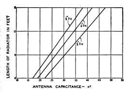
Fig. 15-4 — Graph showing the approximate capacitance of short vertical antennas for various diameters and lengths. These values should be approximately halved for a center-loaded antenna.
