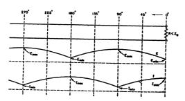
Fig. 3-12 — Standing waves of current and voltage along the line, for R less than Zo.
