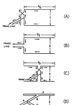
Fig. 4-21 — Parallel-element end-fire array with various methods of feed, showing current distribution. Matching sections for making the transmission line nonresonant, as described in Chapter Three, may be used in the first three cases. The distance  $\mathcal S$  may be selected from Fig. 4-20.
