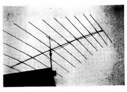
Fig. 9-17 - The log-periodic dipole array (K4EWG).
