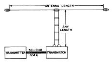
Fig. 6-4 — A center-fed antenna system for multiband use.
