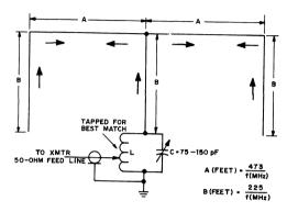
Fig. 16-16 — Bobtail curtain is an excellent low-angle radiator having broadside bidirectional characteristics. Current distribution is represented by the arrows. Dimensions A and B (in feet) can be determined by the formulas. An extensive ground system is not necessary.
