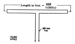
Fig. 2-86 - The folded dipole.
