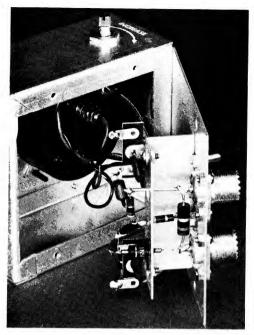
Fig. 17-5 - A 2  $\times$  4  $\times$  4-inch aluminum box is used to house this SWR bridge, which uses the circuit of Fig. 17-4. The variable resistor, R4, is mounted on the side.
