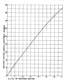
Fig. 3-72 — Inductive reactance (normalized to Zo of matching section), scale at bottom, versus required matching-section length, scale at left. To determine the length in wavelengths, divide the number of electrical degrees by 360. For open-wire line, a velocity factor of 97.5% should be taken into account when determining the electrical length.
