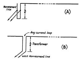
Fig. 5-5  $-\,$  Methods of feeding long single-wire antennas.
