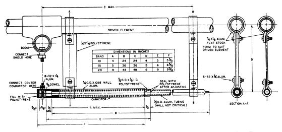
Fig. 9-7 — Constructional details of a gamma-matching section for 52-ohm coax line. The reactance-compensating capacitor is in tubular form. It is made by dividing the gamma rod or bar into two telescoping sections separated by a length of polystyrene tubing, which serves as the dielectric.
