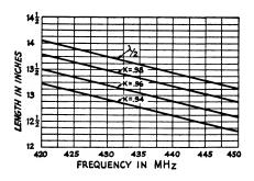
Fig. 11-1 — Frequency vs. length in inches for the 50-, 144-, 220- and 420-MHz bands, for a freespace half wavelength and resonant antenna lengths for various element length/thickness ratios (see Chapter Two). Lengths for values of K other than those given can be found by linear interpolation, e.g., the curve for K=0.97 lies midway between the curves for K=0.96 and 0.98, etc. To find the free-space wavelength used in calculating spacings multiply the length given for  $\lambda/2$  by 2.
