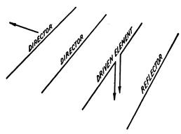
Fig. 4-49 — A four-element antenna system, using two directors and one reflector in conjunction with a driven element.
