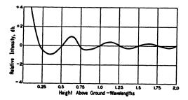
Fig. 2-52 — Gain or loss in decibels because of change in antenna current with radiation resistance, for fixed power input. Perfectly conducting ground is assumed.
