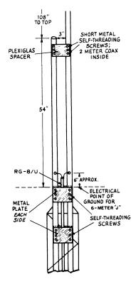
Fig. 11-47 — Details of the 6-meter J pole.
