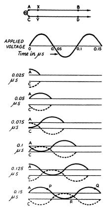
Fig. 3-4 — Instantaneous current along a transmission line at successive time intervals. The frequency is such that the time of one cycle is 0.1 microsecond.
