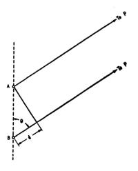
Fig. 2-18 — Graphical construction to determine the relative phase, at a distant point, of waves originating at two antennas, A and B. The phase is determined by the additional distance, d, that the wave from B has to travel to reach the distant point. This distance will vary with the angle that the direction to P makes with the axis of the antenna system,  $\theta$ .
