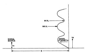
Fig. 17-22 — The vertical profile, or plot of signal strength versus test-antenna height, for a fixed height of the signal source above ground and at a fixed distance. See text for definitions of symbols.
