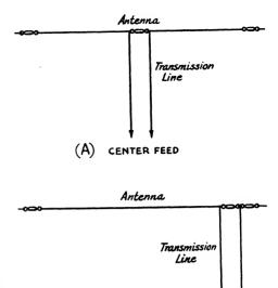
Fig. 346- Center and end feed as used in simple antenna systems.
