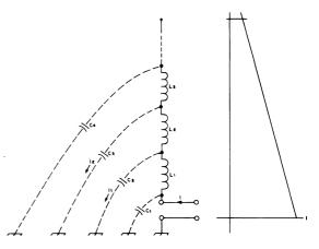
Fig. 15-5 — A circuit approximation of a simple whip over a perfectly conducting ground-plane. The shunt capacitance per unit length gets smaller as the height increases, and the series inductance per unit length gets larger. Consequently, most of the antenna current returns to the ground plane near the base of the antenna, giving the current distribution shown on the right.
