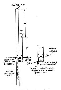
Fig. 11-46 — Details of the 2-meter J pole.
