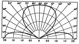
Fig. 2-38 — Vertical dipole antenna with center 1/2 wavelength high.
