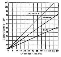
Fig. 2-80 — Capacitance of sphere, disk and cylinder as a function of their diameters. The cylinder length is assumed equal to its diameter.
