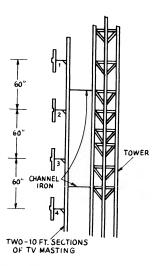
Fig. 11-48 — Spacing and arrangement of the four phased half-wavelength dipoles.
