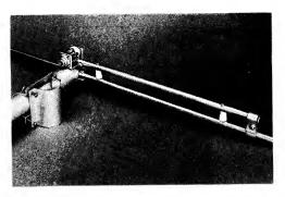
Fig. 11-15 — Typical gamma-match construction. The variable capacitor, 50 pF, should be mounted in an inverted plastic cup or other device to protect it from the weather. The gamma arm is about 12 inches long for 50 MHz, 5 inches for 144 MHz.
