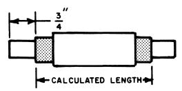
4) Using single-edge razor blade, trim insulation leaving 1/16" to 1/8" remaining.
