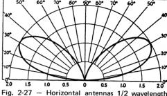
Fig. 2-27 - Horizontal antennas 1/2 wavelength
