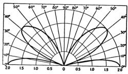
Fig. 2-39 — Vertical dipole antenna with center 3/4 wavelength high.
