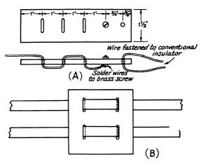
Fig. 13-6 — A — Insulator for ends of folded dipoles, or multiple dipoles made of 300-ohm ribbon. B — A method of suspending one ribbon dipole from another in a multiband dipole system.
