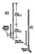
Fig. 11-3 — Two versions of the "J" antenna, used in mobile applications or in vertical arrays where parasitic elements are rotated around a fixed radiator.
