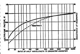
Fig. 2-4 — The solid curve shows the factor, K, by which the length of a half wave in free space should be multiplied to obtain the physical length of a resonant half-wave antenna having the length/diameter ratio shown along the horizontal axis. The broken curve shows how the radiation resistance of a half-wave antenna varies with the length/diameter ratio.
