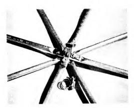
Fig. 10-5 — Construction details for the top hat. For a diameter of 7 feet, half-inch aluminum tubing is used. The hose clamp is of stainless steel and available at Sears. The rest of the hardware is aluminum.
