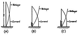
Fig. 2-72 — Current and voltage distribution on a grounded quarter-wave antenna (A) and on successively shorter antennas loaded to resonate at the same frequency.
