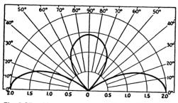
Fig. 2-37 — Vertical dipole antenna with center 3/8 wavelength high.
