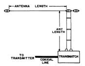
Fig. 6-3 — An end fed antenna for multiband use.
