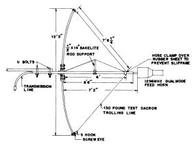
Fig. 12-11 — Side view of the stressed parabolic dish.
