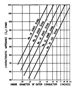
Fig. 3-32 — Characteristic impedance of typical air-insulated coaxial lines.
