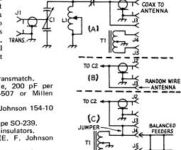
Fig. 6-7 — Circuit diagram of the Transmatch.
