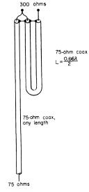
polyethylene-insulated coaxial and parallel lines, respectively. The exact length for a matching section can be determined experimentally, if desired, by shorting one end of the line, coupling it to a calibrated grid-dip oscillator, and then trimming the line length until the grid-dip meter shows it to be resonant at the desired frequency.
