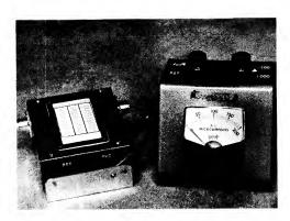
Fig. 17-8 — The rf wattmeter consists of two parts, the rf head (left), and the control/meter box (right). The paper scale affixed to the rf head contains the calibration information which appears in Fig. 17-9.
