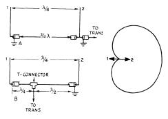
Fig. 8-9 — Two methods of feeding the phased verticals.
