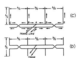
Fig. 16-6 — Methods of feeding three- and fourelement broadside arrays with parallel elements.
