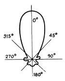
Fig. 4-65 — Measured radiation pattern for the lowest frequency band (14 MHz) of a 12-element 13-30 MHz log-periodic dipole array. For its design parameters,  $\tau = 0.9$  and  $\sigma = .05$ . The measured front-to-back ratio is 14.4 dB at 14 MHz, and increases to 21 dB at 28 MHz.
