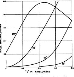
Fig. 11-37 — Feed impedance of the driven element in a corner-reflector array, for various corner angles of 180 (flat sheet), 90, 60 and 45 degrees.
