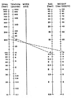
Fig. 13-2 — Nomograph for determining wire sag. (K1AFR.)
