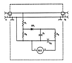
Fig. 17-1 — Rf voltmeter for coaxial line.
