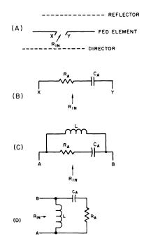
Fig. 3-70 — For the Yagi antenna shown at A, the input impedance at its operating frequency is represented at B, if the driven element is shorter than its resonant length. By adding an inductor, as shown at C, a low value of RA is made to appear as a higher impedance at terminals AB. At D, the diagram of C is redrawn in the usual L-network configuration.
