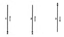
Fig. 4-6 - Illustrating phasing of currents in antenna elements.
