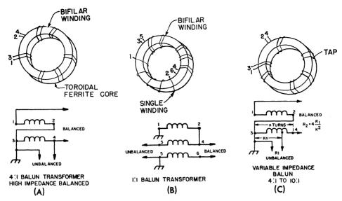
Fig. 3-45 - Basic broad-band balun transformers.
