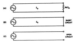
Fig. 3-7 — Mismatched lines. A — termination not equal to Zo; B — short-circuited line; C — open-circuited line.
