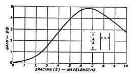
Fig. 4-16 — Power gain as a function of the spacing between two parallel elements operated in phase (broadside).
