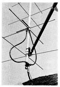
Fig. 12-1 — This vhf crossed Yagi antenna design by KH6IJ was presented in January 1973 *QST*. Placement of the phasing harness and T connector is shown in the lower half of the photograph. Note that the gamma match is mounted somewhat off of element center for better balance of rf voltages on elements.
