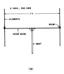
Fig. 11-43 — Methods of mounting Yagi antennas with the elements vertical. The boom-to-mast joint may be strengthened by a gusset plate. If the arrays are large enough to require diagonal bracing, such bracing should be of nonconducting material where it is close to the elements.
