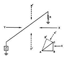
Fig. 5-9 - Nonresonant long-wire antenna.
