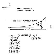
Fig. 12-16 — Parabolic template for 12-foot, 3-inch dish.
