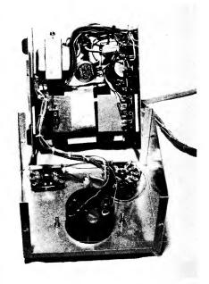
Fig. 14-7 — Inside view of the Hy-Gain control box.
