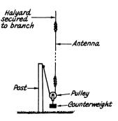
Fig. 13-22 — Counterweight for a vertical antenna suspended from an overhanging tree branch.
