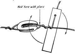
Fig. 13-25 - Simple lever for twisting solid guy wires in attaching strain insulators.
