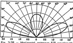
Fig. 2-28 Horizontal antennas 5/8 wavelength high.
