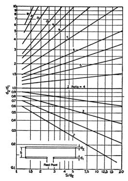
Fig. 2-87 — Impedance step-up ratio for the two-conductor folded dipole, as a function of conductor diameters and spacing. Dimensions  $d_1$ ,  $d_2$  and S are shown in the inset drawing. The step-up ratio, r, may also be determined from:
