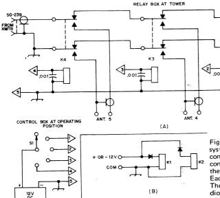
Fig. 8-15 — Schematic diagram for sloper control system. All relays are 12-volt dc, dpdt with 8-A contact ratings. In A, the basic layout, excluding control cable and antennas. Note that the braid of the coax is also open-circuited when not in use. Each relay is bypassed with .001- $\mu F$  capacitors. The power supply is a low-current type. In B, diodes are used to reduce the number of control wires when using dc relays. See text.
