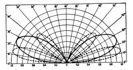
Fig. 4-29 — Vertical pattern of the four-element antenna of Fig. 4-27 when mounted horizontally. Solid curve, height 1/2 wavelength; broken curve, height 1 wavelength. Fig. 4-28 gives the horizontal pattern.
