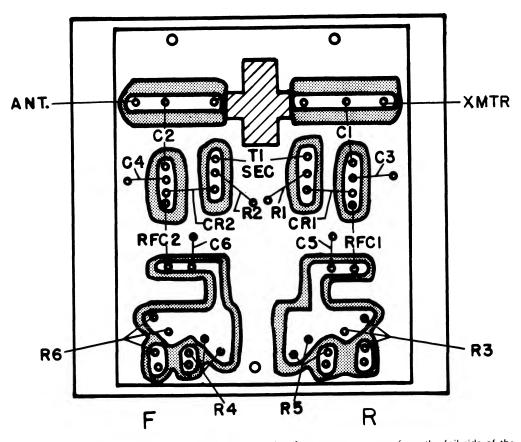
Fig. 17-11 — Etching pattern and parts layout for the rf wattmeter, as seen from the foil side of the board. The etched-away portions of the foil are shown as darkened areas in this drawing. The area represented with diagonal lines is to be cut out for the mounting of T1.
