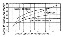
Fig. 4-53 — Gain of long Yagi antennas as a function of overall length. The antenna consists of a driven element, a single reflector spaced approximately one-fourth wavelength from the driven element, and a series of directors spaced as described in the text. The three curves represent the results of three independent studies.
