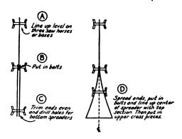
Fig. 13-24 — Method of assembling the "A-frame" mast.
