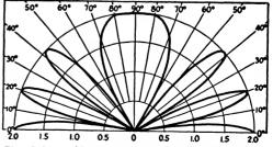
Fig. 2-41 - Vertical dipole antenna with center 1-1/2 wavelengths high.
