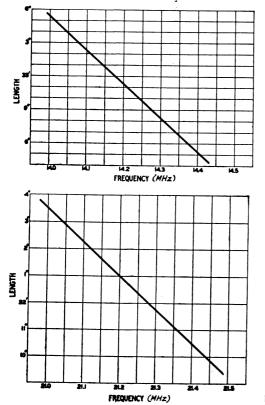
described in Chapter Eight, it is ordinarily useful only on the band for which it is designed. Suitable lengths for wire antennas are given in Fig. 9-1, and Fig. 3-53 should be referred to if feeder resonances are to be avoided. Vertical antennas (and the ground plane in particular) can be used at these frequencies and will give good low-angle radiation. However, with a vertical receiving antenna, manmade noise pickup is likely to be greater than with a horizontal antenna.
