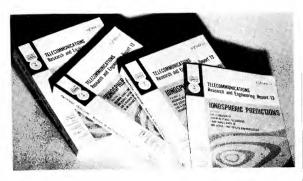
Fig. 1-12 - With these four volumes, frequency estimations for sky-wave signals can be made manually for any month of any year. The only other information required is the Zurich smoothed relative sunspot number for the period of interest.
