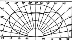
Fig. 2-26 - Horizontal antennas 3/8 wavelength
