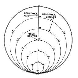
Fig. 3-16  $\,-\,$  Resistance circles of the Smith Chart coordinate system.
