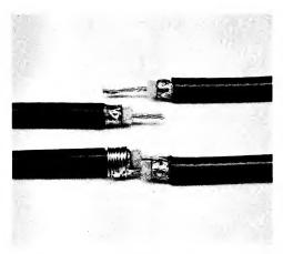
Fig. 11-52 — This shows the prepared end of one of the coax sections and also the method of joining two sections together.
