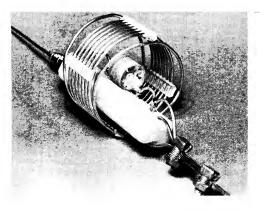
Fig. 6-14 — Easily constructed trap for wire antennas (W2CYK). The ceramic insulator is 4-1/4 inches long (Birnbach 668). The clamps are small service connectors available from electrical supply and hardware stores (Burndy KS90 Servits).
