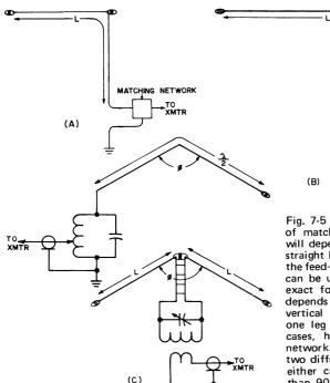
radiation efficiency drops very rapidly. The drawings in Fig. 7-4 show some of the configurations of the various antenna types discussed.
