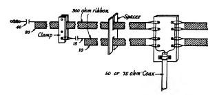
Fig. 6-11 — Sketch showing how the Twin-Lead multiple-dipole antenna system is assembled. The excess wire and insulation are stripped away.
