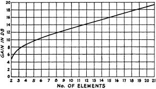
Fig. 4-51 — Optimum length of Yagi antenna as a function of number of elements.
