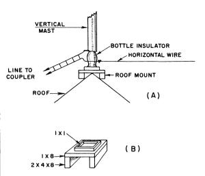
Fig. 6-19 - One method of mounting the vertical section on a rooftop. The mounting base dimensions can be adjusted to fit the pitch of the roof. The 1 x 1 pieces should fit snugly around the bottom of the bottle to keep it from shifting position.
