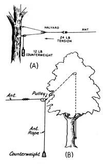
Fig. 13-18 — Methods of counterweighting to minimize antenna movement. The method at A limits the fall of the counterweight should the antenna break. It also has a 2 to 1 mechanical advantage, as indicated. The method at B has the disadvantage that the point of support in the tree must be higher than the end of the antenna.
