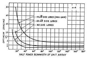
Fig. 4-55 — Optimum stacking spacing for four-unit arrays.
