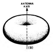
Fig. 2-12 — At A, directive diagram of an elementary doublet in the plane containing the wire axis. The length of each dash-line arrow represents the relative field strength in that direction. At B, the solid pattern of the same antenna. These same diagrams apply to any antenna considerably less than a half wavelength long.
