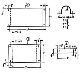
Fig. 11-31 — Detail drawings of the clamps used to assemble the all-metal 2-meter array. A, B and C are before bending into "U" shape. The right-angle bends should be made first, along the dotted lines as shown, then the plates may be bent around a piece of pipe of the proper diameter. Sheet stock should be 1/16-inch or heavier aluminum.
