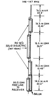
Fig. 11-50 — Basic details of the coaxial-collinear antenna. See fig. 11-9A for balun details.
