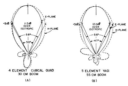
Fig. 5-59 — Measured patterns of 4-element quad and 5-element Yagi antennas, showing approximately equivalent beamwidths. Measurements made on model antennas at 440 MHz by W7ZQ.
