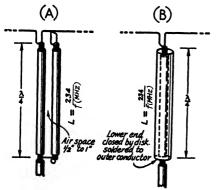
Fig. 3-57 — Methods of balancing the termination when a coaxial cable is connected to a balanced antenna.
