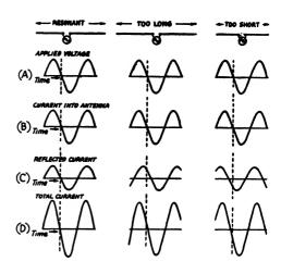
Fig. 2-6 — Current flow in resonant and offresonant antennas. The initial current flow, B, caused by the source of power, is in phase with the applied voltage, A. This is the outgoing current discussed in the text. The reflected current, C, combines with the outgoing current to form the resultant current, D, at the input terminals of the antenna.
