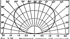
Fig. 2-25 Horizontal antennas 1/4 wavelength high.
