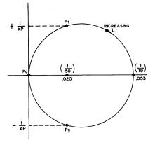
Fig. 15-7 — Admittance diagram of the RLC circuit consisting of the whip capacitance, radiation resistance and loading coil discussed in text. The horizontal axis represents conductance, and the vertical axis susceptance. The point Po is the input admittance with no whip loading inductance. Points P1 and P2 are described in the text.
