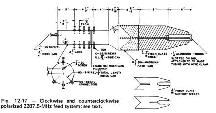
launches an ordinary linear wave. The small cans are "Scotts Oats" type from Scotland or "Camp" drain cleaner cans from the U.S., 3-3/4 inches ID. The large can is a one-gallon paint can, 6-1/2 inches ID. The 30-degree section is galvanized sheet metal. Tabs on each end add strength and make soldering the cans together easier.
