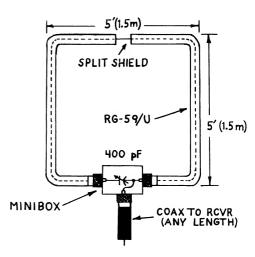
Fig. 7-7 — Schematic diagram of the loop antenna. The dimensions are not critical provided overall length of the loop element does not exceed approximately .04 wavelength. Small loops which are one half or less the size of this one will prove useful where limited space is a consideration.
