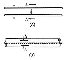
Fig. 3-1 - The two basic types of transmission lines.
