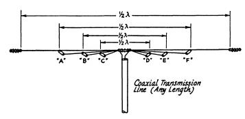
Chapter Three) as shown in Fig. 6-9B. The same balun will transform the impedance to 75 ohms, in cases where the line actually shows a resistive input impedance of 300 ohms.
