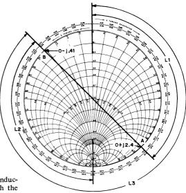
Fig. 3-28 — Smith Chart determination of input impedances for short- and open-circuited line sections, disregarding line losses.
