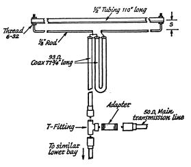
Fig. 11-25 — Details of the driven elements and phasing system used in the 50-MHz stacked array. The folded dipole is set up so that its feed impedance is approximately 400 ohms. Two halfwave baluns and half-wave phasing sections step down to about 100 ohms. The two bays thus connected in parallel may be fed with 50-ohm coax directly.
