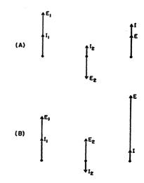
Fig. 3-10 — Incident and reflected components of voltage and current when the line is terminated in a pure resistance not equal to  $Z_0$ . In the case shown, the reflected components have half the amplitude of the incident components. A -R less than  $Z_0$ ; B -R greater than  $Z_0$ .
