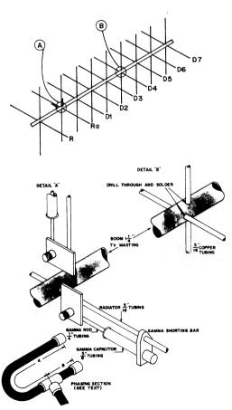
Fig. 12-3 — Construction details of a crossed Yagi antenna.
