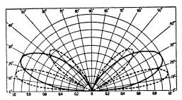
Fig. 4-24 — Vertical pattern of a horizontally polarized two-element end-fire array. Solid curve, height 1/2 wavelength; broken curve, height 1 wavelength.
