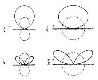
Fig. 2-23 — Effect of the ground on the radiation from a horizontal half-wave antenna, for heights of one-fourth and one-half wavelength. Dashed lines show what the pattern would be if there were no reflection from the ground.
