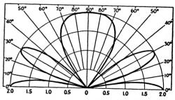
Fig. 2-40 — Vertical dipole antenna with center 1 wavelength high.
