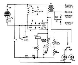
Fig. 14-3 — Diagram of the modified Ham-M rotor-control box. Fixed-value resistors are 1-watt composition. Connections must be broken at the two places marked "X." The shaded lines indicate original wiring and the heavy lines are additions to the original circuit. Parts designations not listed below are for text reference.
