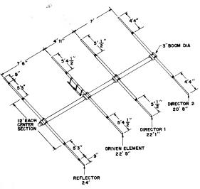
Fig. 9-2 - Overall dimensions for the 4-element 15-meter array.
