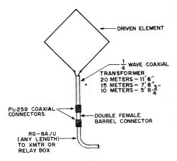
Fig. 9-16 — Showing installation of quarter-wave 75-ohm transformer section.
