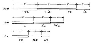
Fig. 9-6 — Suggested proportions for one side of tapered Yagi elements. The other side is identical, of course, and the center section of the element can be a single piece twice as long as the length shown here for the first (largest diameter) section. Appropriate overall element lengths may be determined from the graphs of Fig. 9-5. See Table 14-I for aluminum tubing details.
