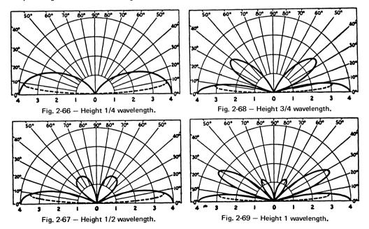
of the free-space pattern of a half-wave dipole by the ground-reflection factor that applies at each wave angle for the antenna height selected, to obtain the resultant relative field strength at each wave angle. The solid pattern in each case is formed by rotating the plane pattern about the 90-degree axis of the graph.
