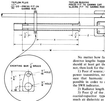
Fig. 12-4 - Gamma-match construction details.
