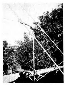
Fig. 12-5 — Two individual Yagis are mounted with the elements at  $90^\circ$  to each other. Elevation and azimuth movements are provided by two TV rotators.
