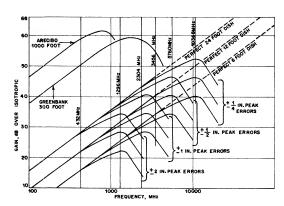
Fig. 12-14 — Parabolic-antenna gain versus size, frequency, and surface errors. All curves assume 60-percent aperture efficiency and 10-dB power taper. Reference: J. Ruze, British *IEE*.
