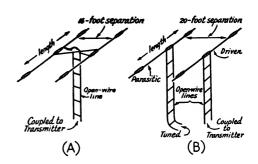
Optimum directivity occurs at right angles to the plane of the loop, or in more simple terms, broadside from the loop. Therefore, one should try to hang the system from available supports which will enable the antenna to radiate the maximum amount in some favored direction.
