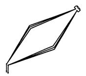
Fig. 5-17 — Three-wire rhombic antenna. Use of multiple wires improves the impedance characteristic of a nonresonant rhombic and increases the gain somewhat.
