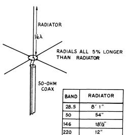
overcome this problem because the horizontal ground plane is an effective shield between the antenna and mast. The fundamental principles of the ground plane are given in Chapter Two, and matching it to commonly available feed lines is discussed in Chapter Three.
