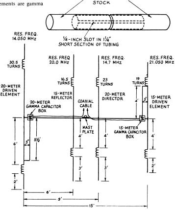
Fig. 10-12 - Constructional details for the 20and 15-meter beam. The coils for each side of the element are identical. The gamma capacitors are each 140-pF variable units manufactured by E.F. Johnson Co. The capacitors are insulated from ground within the container. Since the antenna is one-half size for each band, the tuning is somewhat critical. builder is encouraged to follow carefully the dimensions given here.
