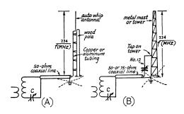
without decreasing the low-angle radiation. The vertical member can be a length of self-supporting tubing at the top of a short mast, and the radials can be lengths of wire used also to support the mast. The radials do not have to be exactly horizontal, as shown in Fig. 8-5.
