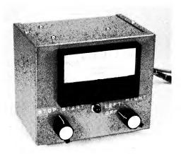
Fig. 14-5 — Front view of the Hy-Gain control box.
