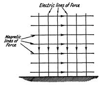
Fig. 1-1 — Representation of the magnetic and electric fields of a vertically polarized plane wave traveling along the ground. The arrows indicate instantaneous directions of the fields for a wave traveling perpendicularly out of the page toward the reader. Reversal of the direction of one set of lines reverses the direction of travel. There is no change in direction when both sets are reversed. Such a dual reversal occurs, in fact, once each half cycle.
