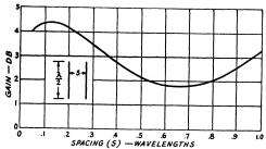
Fig. 4-20 — Gain of an end-fire array consisting of two elements fed 180 degrees out of phase, as a function of the spacing between elements. Maximum radiation is in the plane of the elements and at right angles to them at spacings up to 0.5 wavelength, but the direction changes at greater spacings.
