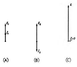
Fig. 3-9 — Voltage and current at the end of an open-circuited line. A — outgoing voltage and current; C — resultant.
