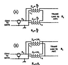
Fig. 3-43 — Air-core balun coils as an impedance-matching device for coupling between balanced and unbalanced lines. A properly designed set of coils will work over the 3.5-30-MHz range without adjustment. However, only the fixed impedance ratios shown are available and the input impedance of the transmission line must be a pure resistance that will match the Z0 of the coils.
