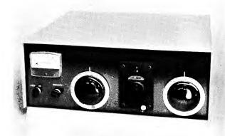
Fig. 6-5 — The universal Transmatch shown here will couple a transmitter to almost any antenna system. The meter is part of an optional built-in SWR indicator. Suitable indicators for inclusion, if the builder desires, are given in Chapter Seventeen.
