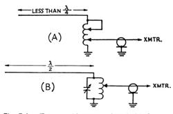
Fig. 7-4 — Two matching networks suitable for use with random-length horizontal (or vertical) wire antennas. If the electrical length is less than 1/4 wave, the input impedance will be equivalent to a resistance in series with a capacitive reactance and the circuit at A should be used. For lengths in the vicinity of 1/2 wave, the input impedance will be fairly high and may have reactances which are either inductive or capacitive. For this case, the parallel-tuned circuit in B should be used.
