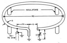
Fig. 10-8 — RD =  $0.078\lambda(28^\circ)$ ; SP =  $0.11D(2.5^\circ)$ ; FP = 0.25SP (see Note 1); C = (see Note 2); D = (see Note 3); G = (see Table 10-I). *Notes*: (1) Actual dimension must be found experimentally. (2) Value to resonate the antenna to the operating freq. (3) D ranges upward from 1/2". The larger D is, the higher the efficiency is. Use largest practical size, e.g., 1/2" for 10 meters, 5" or 6" for 80 or 160 meters.
