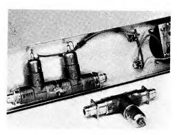
Fig. 17-15 — Two versions of the line sampler. The single unit described in detail here is in the foreground. Two sections in a single assembly provide for monitoring forward and reflected power without probe reversal.
