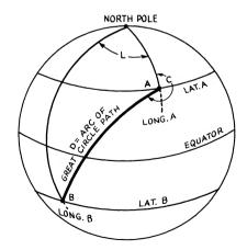
Fig. 18-5 - Showing the various terms used in the equations for determining bearing and distance. North latitudes and west longitudes are taken as positive, while south latitudes and east longitudes are taken as negative.
