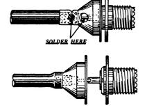
5) Slide hood over braid. Bring receptacle flush against hood. Solder hood to braid and conductor to contact sleeve through solder holes as illustrated. Tape junction if necessary. (For UG-372/U.)
