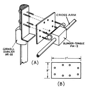
Fig. 12-8 — The method of mounting two rotators together. A pair of PM-2 rotators may also be used. The adapter plate (B) may be fabricated from 1/4-inch-thick aluminum stock, or a ready-made plate is available from Blonder-Tongue.
