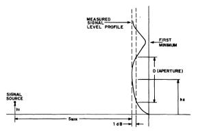
Fig. 17-23 — Sample plot of a measured vertical profile.
