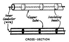
Fig. 3-31 — Construction of air-insulated coaxial lines.
