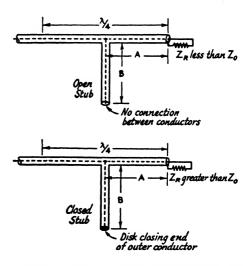
Fig. 3-75 — Open and closed stubs on coaxial lines.
