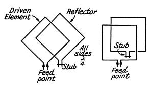
Fig. 4-57 — The basic quad antenna, with driven loop and reflector loop. The loops are electrically one wavelength in circumference (1/4 wavelength on a side). Both configurations shown give horizontal polarization; for vertical polarization, the driven element should be fed at one of the side corners in the arrangement at the left, or at the center of a vertical side in the "square" quad at the right.
