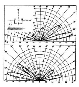
Fig. 4-39 — Vertical patterns of a horizontally polarized two-element array under the conditions given in Fig. 4-38. These patterns are in the vertical plane at right angles to the antenna elements.
