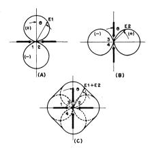
Fig. 12-2 — Radiation patterns looking head-on at dipoles.
