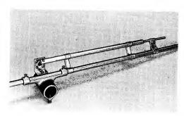
Fig. 11-22 — Gamma matching section using tubular capacitor. The sheet-aluminum clip at the right is moved along the driven element for matching. The small rod can be slid in and out of the 15-inch tube for adjustment of series capacitance. The rod should be about 14 inches long.
