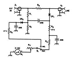
Fig. 17-4 — Resistance bridge for SWR measurement. Capacitors are disk ceramic. Resistors are 1/2-watt composition except as noted below. CR1, CR2 — Germanium diode, high back-
