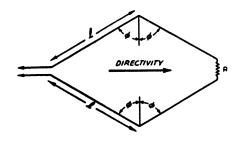
Fig. 5-12 — The nonresonant rhombic antenna.
