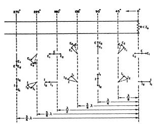
Fig. 3-11 — Incident and reflected components at various positions along the line, together with resultant voltages and currents at the same positions. The case shown is for R less than Zo.
