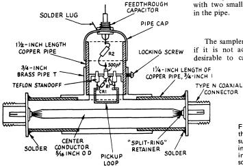
Fig. 17-14 — Cross-section view of the line sampler. The pickup loop is supported by two Teflon standoff insulators. The probe body is secured in place with one or more locking screws through holes in the brass T.
