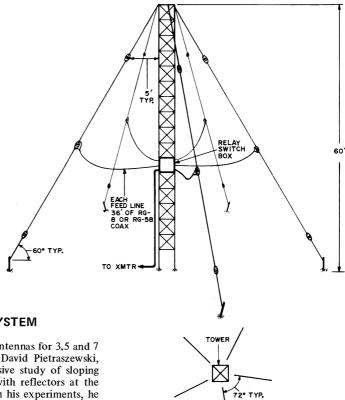
Fig. 8-12 — Five sloping dipoles suspended from one support. Directivity and forward gain can be obtained from this simple array. Top view shows how the elements should be spaced around the support.
