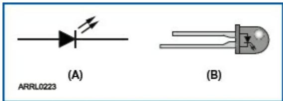
Figure 5.14 — The schematic symbol for an LED is shown at A. B is a drawing of a typical LED case style.
