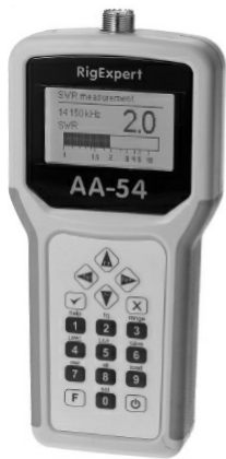
Figure 9.37 — An antenna analyzer, such as this RigExpert AA-54, consists of a tunable signal source, a frequency counter, an impedance bridge, and displays — all microprocessor controlled. The analyzer displays impedance, SWR, and frequency.
