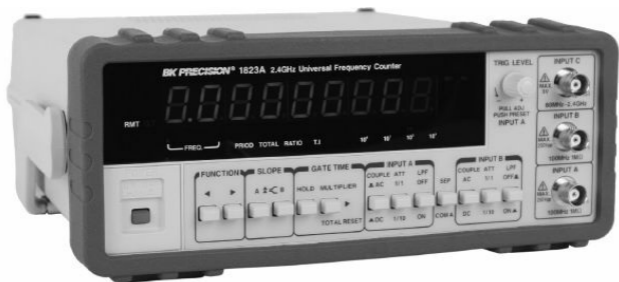
Figure 7.2 — Typical frequency counter used by hams for troubleshooting and construction. Many lab-grade counters are available as surplus or used equipment. Frequency counters are also available in kit form and as new equipment. [Courtesy of B&K Precision]
