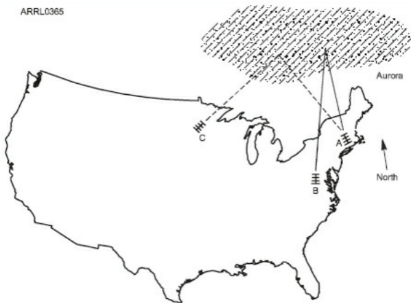
Figure 10.13 — To use auroral propagation, stations point their antennas toward the Geomagnetic North Pole. Station A may have to beam west of north to work station C.
