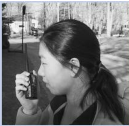
Figure 4.A — To get the best range from a handheld radio, hold it so that the antenna is vertical. This aligns your antenna with those of a repeater or another handheld user. Also, turn the microphone slightly away from your face when talking so that your breath does not blow directly into it.
