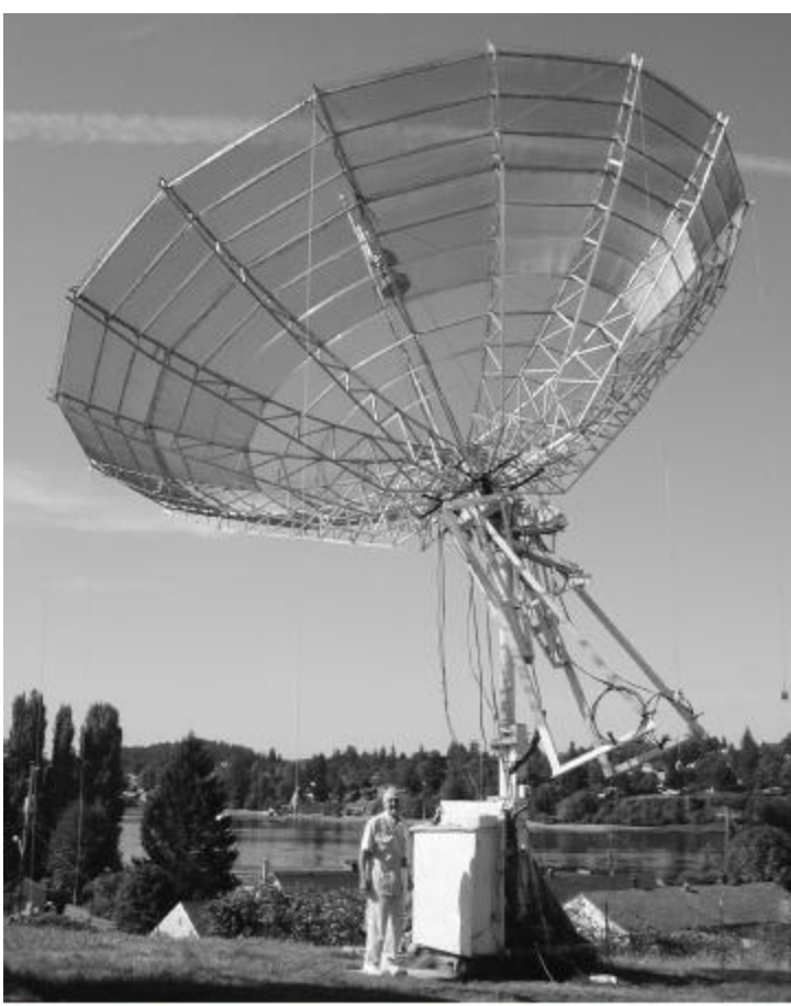
Figure 4.14 — The 10-meter diameter dish shown on the left was used on 1296 MHz to bounce signals off the moon and for long-distance terrestrial contacts. N7CFO's much smaller dish (right) operates on 10 GHz and is portable enough to be taken on contest outings.
