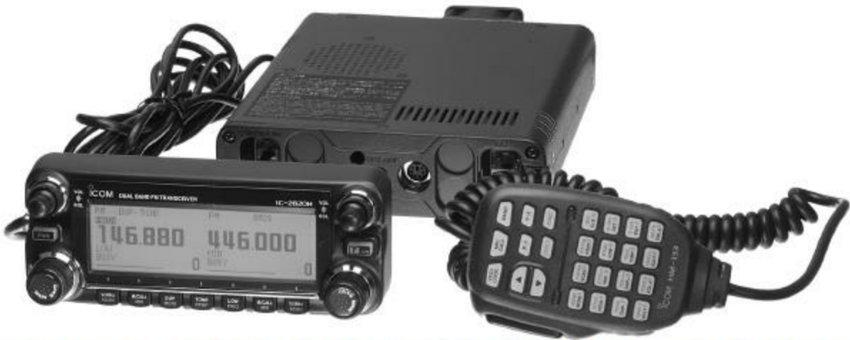
Some transceivers include the ability to separate the front panel (the “control head”) from the rest of the unit for easier mobile installations.
