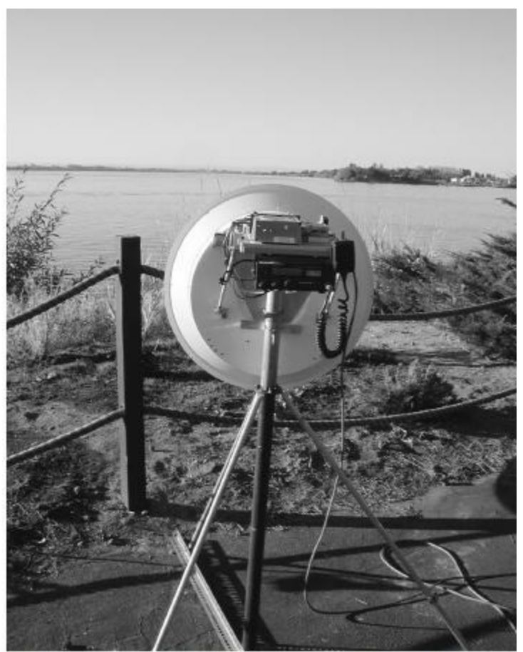
Figure 4.14 — The 10-meter diameter dish shown on the left was used on 1296 MHz to bounce signals off the moon and for long-distance terrestrial contacts. N7CFO's much smaller dish (right) operates on 10 GHz and is portable enough to be taken on contest outings.
