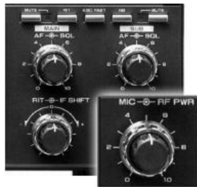
Figure 5.3 — The maximum output power of HF transceivers is set by an RF PWR knob. This control does not affect MIC GAIN or other audio settings. On mobile rigs, output power is varied between several preset levels with a button or key.
