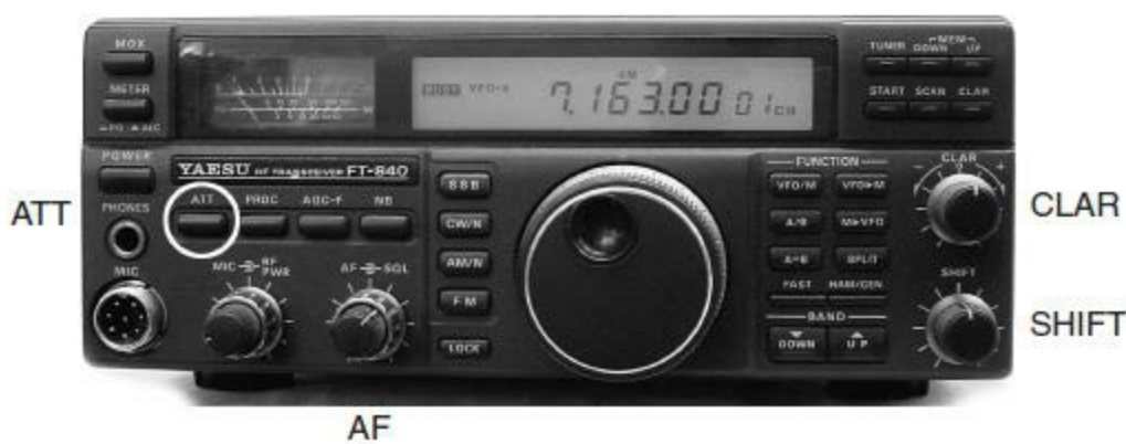
Figure 5.7 — The front panel of this Yaesu FT-840 transceiver has most of the receiver controls you'll use every day. AF GAIN (labeled AF) controls volume. CLAR (RIT) and SHIFT vary the receiver frequency without changing your transmit frequency. ATT adds attenuation to reduce the strength of very strong signals.
