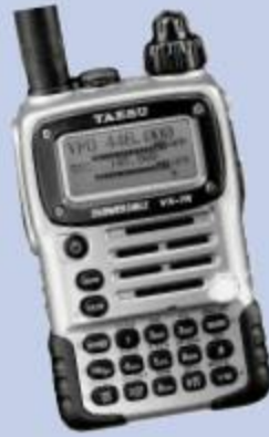
Figure 5.2 — Because front-panel space is limited, some buttons and keys can perform more than one function. A control or function key causes the alternate functions to be used. On the VX-7R handheld a single MON-F key controls both alternate functions and writing information into the radio's memories.
