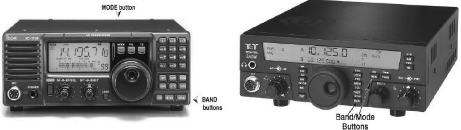
Figure 5.1 — The frequency and mode controls are shown for a pair of HF radios, the Icom IC-718 (left) and the Ten-Tec Eagle (right). Frequency within a band can be adjusted with the large tuning knob or by the numeric keypad. If a computer is connected to the radio, frequency may be changed by the computer software. Pressing the MODE key switches between CW, USB and LSB and other available modes.
