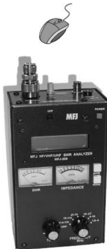
Figure 4.18 — The popular MFJ series of antenna analyzers are used to adjust and troubleshoot antenna systems. The instrument contains a low-power signal source with an adjustable frequency and an SWR meter. The LCD display shows the operating frequency and information about the antenna impedance. The meters show SWR and feed point impedance.
