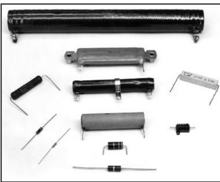
Figure 3.7 — This photograph shows some of the many types of resistors. Large, power resistors are at the top of the photo. The small resistors are used in low-power circuits.
