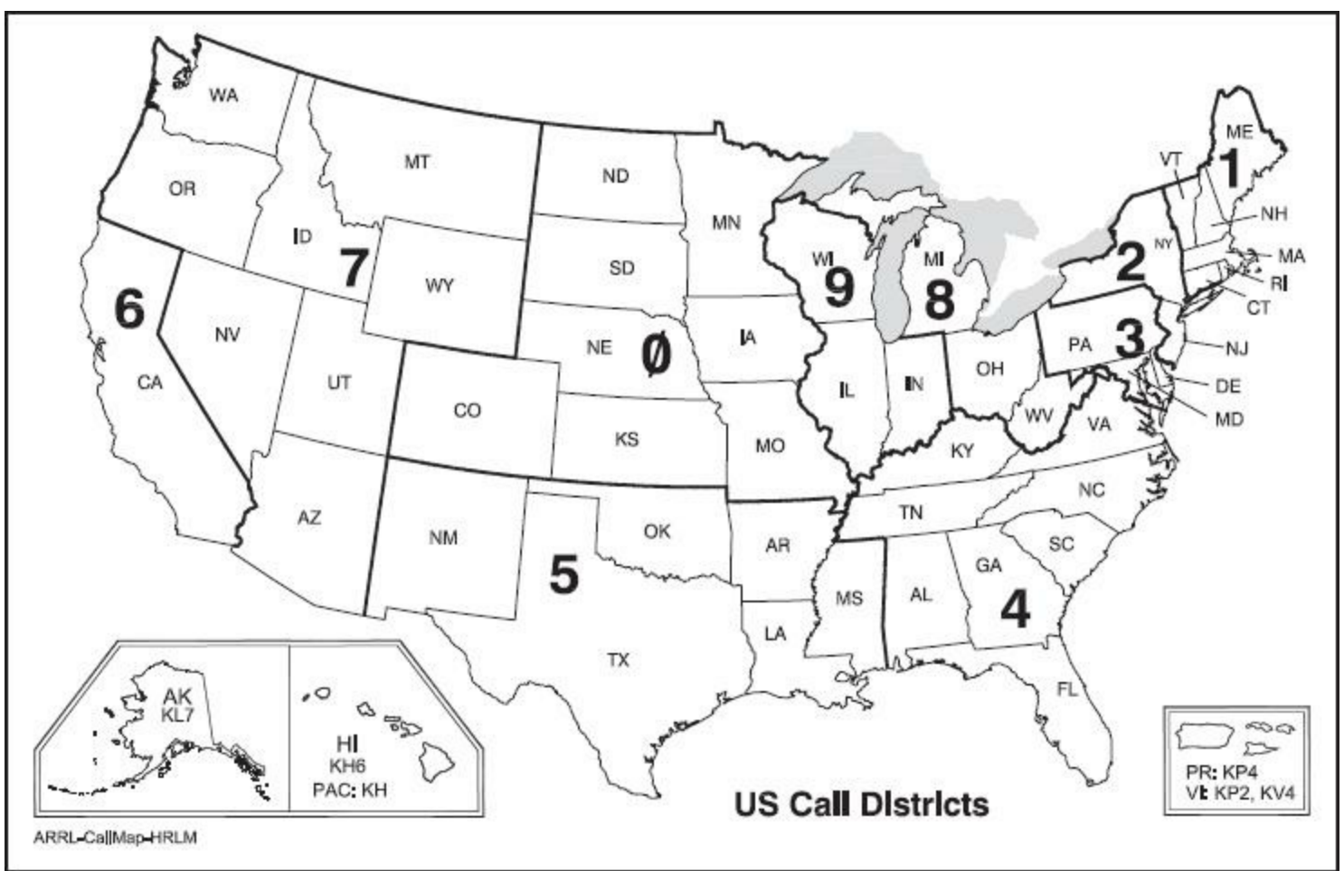
Figure 7.6 — There are 10 US call districts in the continental United States. When an amateur passes their initial license exam, the numeral of the district in which he or she resides becomes part of their assigned call sign. Alaska and the US possessions in the Pacific and Caribbean form three more districts and have calls with unique prefixes.
