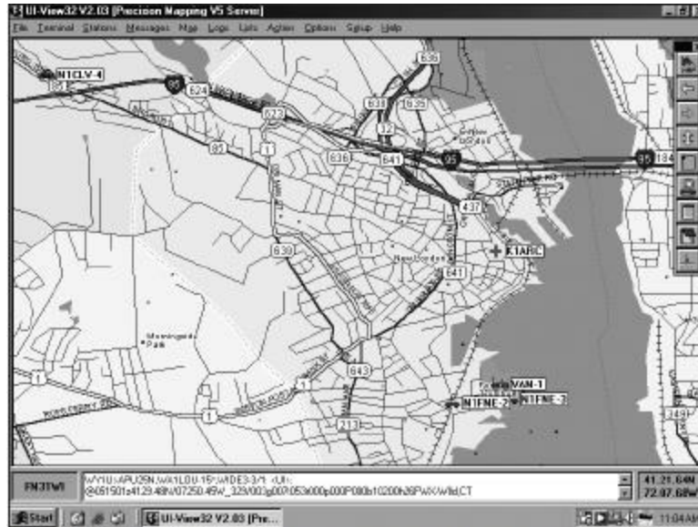
The Automatic Packet Reporting System (APRS) was invented by hams to show location and travel path by using ham radio.
