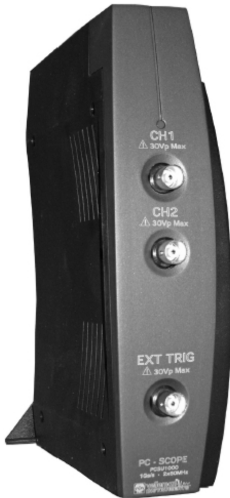
Figure 1.4 — Today's oscilloscopes look more like this. This one is small, fairly low cost and very capable, though it requires a computer and accompanying software for processing, control and display of measured waveforms.
