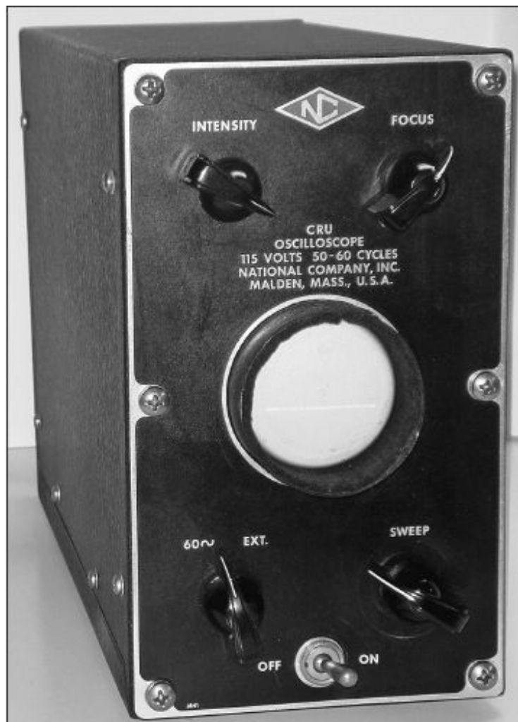
Figure 2.3 — After World War II, National came out with a new scope, featuring a larger tube. [Photo courtesy of Chuck at myvintagetv.com]
