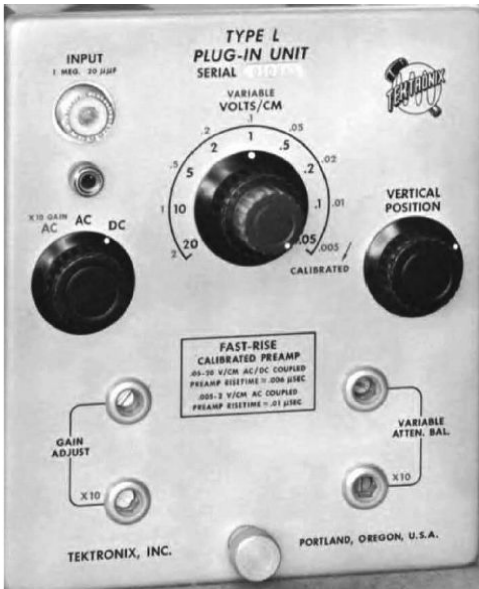
Figure 6.3 —This vintage Tektronix FAST-RISE plug-in front end provides very fast response to rising and falling pulse edges, useful for digital information where the pulse edges are important.
