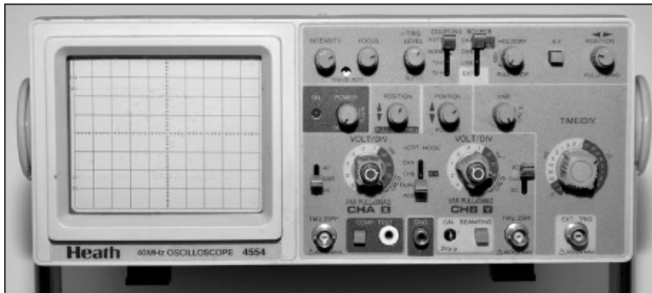
Figure 2.9 — In addition to Tektronix, other manufacturers sold lower cost solid state scopes with excellent performance specifications. [Photo courtesy of Tim Walker, W1GIG]
