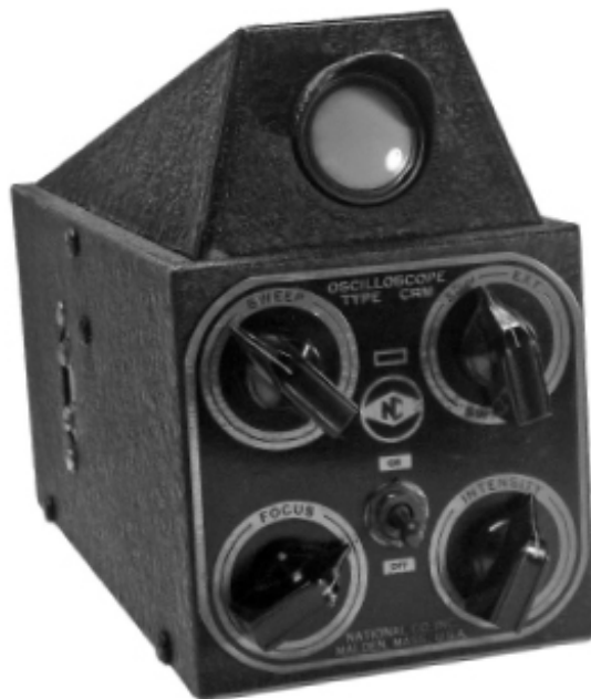
Figure 2.2 — The basic controls on this very early commercial oscilloscope, sold by National Radio, are recognizable today. [Photo courtesy of Chuck at myvintagetv.com]
