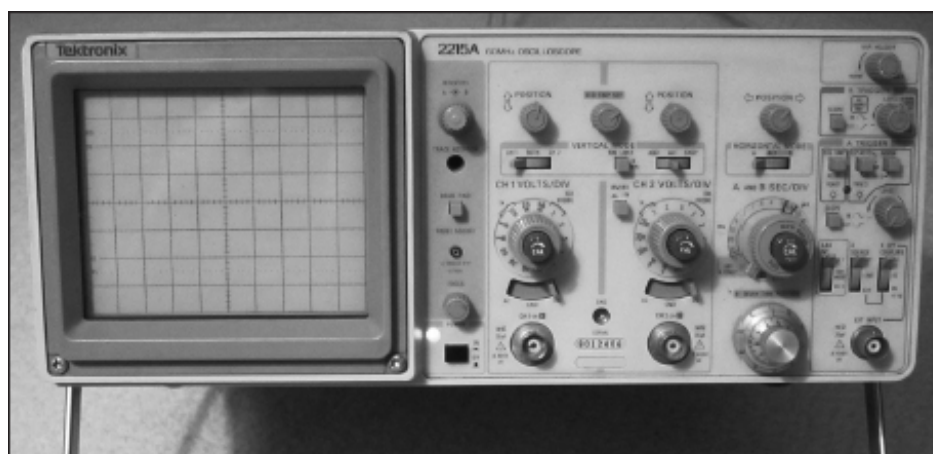
Figure 2.8 — The vacuum tube lab scopes were replaced by solid state lab scopes weighing perhaps one-fifth of the weight of their predecessors and requiring a tenth of the ac power. [Photo courtesy of Rich Roznoy, K10F]
