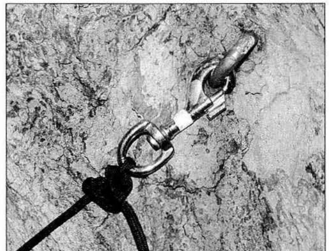
A carabineer and an eyelet screwed into a tree trunk can make a good anchor for an antenna rope.
