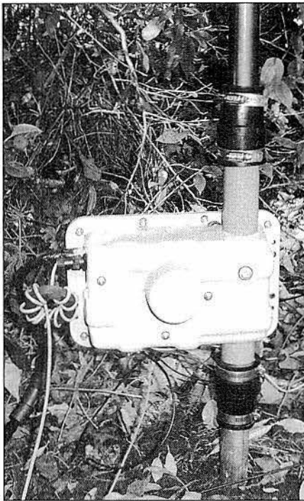
The Fluidmotion SteppIR vertical antenna adjusts its length by using an electric motor at the base to raise or lower a beryllium tape within a fiberglass tube. www.steppir.com
