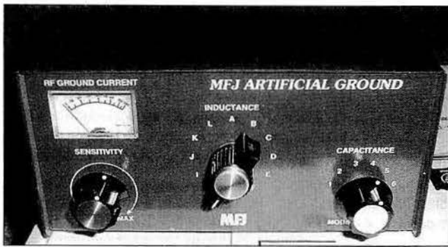
Figure 3.26 — The MFJ-931 “Artificial Ground” by MFJ Enterprises “tunes” the counterpoise wire in end-fed installations. The MFJ-931 connects between the antenna tuner ground and the counterpoise wire.
