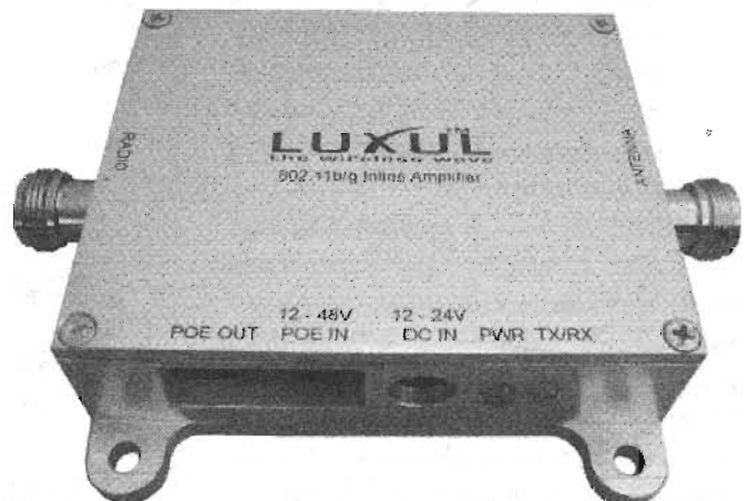
Figure 7-8—A typical bi-directional amplifier for HSMM applications. This unit delivers 1 W output.
