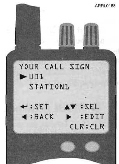
Figure 4-9—"STATION1" programmed into memory U01.
