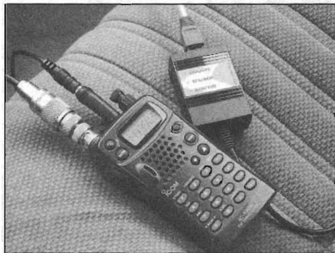
A handheld radio can be turned into an APRS tracker by adding a GPS receiver and a tracking TNC.
