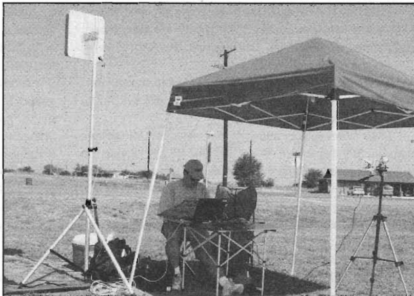
Figure 7-2—N500M and the North Texas Microwave Society have used RooTenna-based systems for public service activities. The RooTenna is the square housing atop the support mast.
