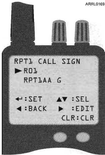
Figure 4-10— “RPT1AA G” programmed into memory R01.
