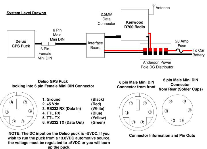
Many will wish to cut off the connector on the puck and wire directly to the interface they are building. Color code and pin out for the puck wiring is provided above.
