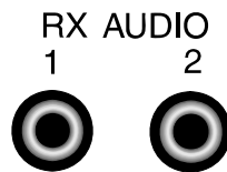
Figure 3-1 Receive audio connections to the DSP.
