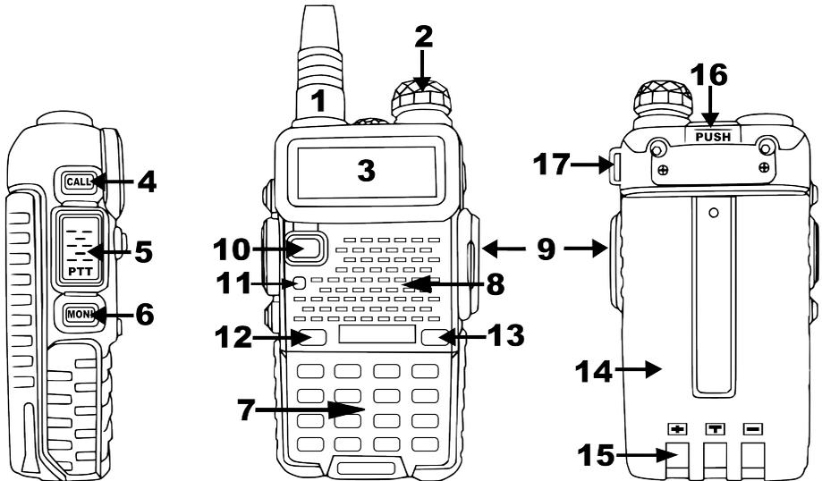
1. Antenna, see [the section called “Assembly”](#) for details.
