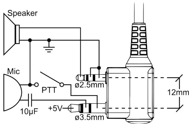
The Kenwood 2-pin connector has one 3.5mm TRS plug, and one 2.5mm TS plug, spaced 12mm apart.
