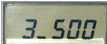
Standard LCD Display showing frequency, 3\_500 translates to 433.500.
