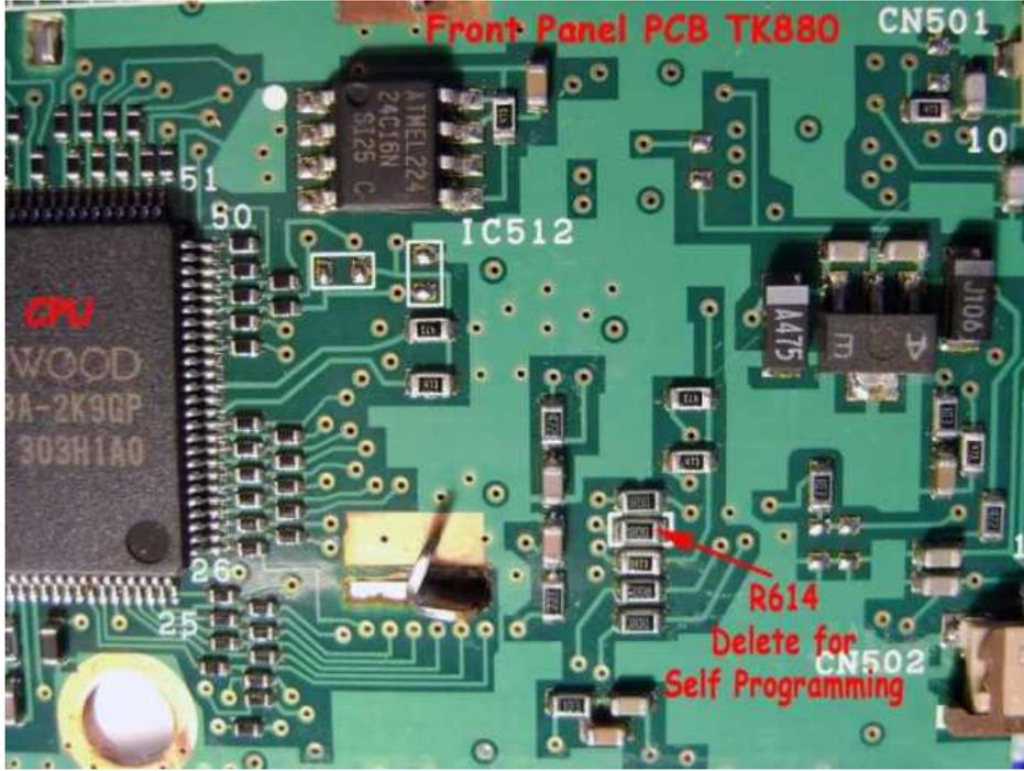
After that, the radio channels can be programmed directly by front panel keys.
