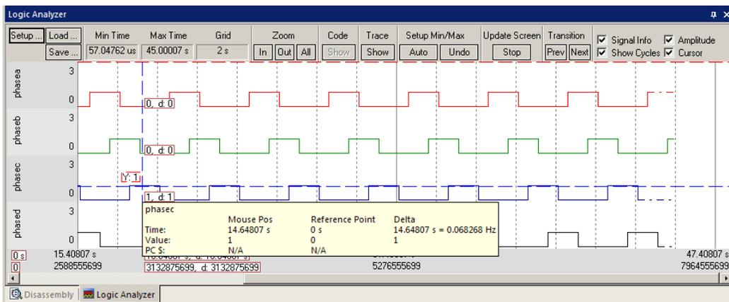
13. Select Signal Info and Show Cycles. Click to mark a place move the cursor to get timings. Place the cursor on one of the waveforms and get timing and other information as shown in the inserted box labeled phasec:
