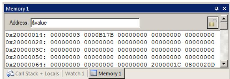
**TIP:** No CPU cycles are used to perform these operations. See the next page “How It Works” for an explanation on how DAP functions.
