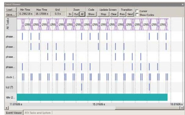
The data is updated while the program is running. No instrumentation code needs to be inserted into your source. You will find this feature very useful ! Remember, RTX with source code is included with all versions of MDK.
