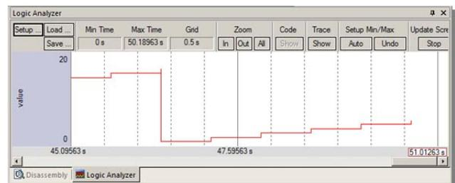
Shown above right is the Logic Analyzer window displaying the variable `value` trigger point of 0x5.
