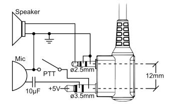
The Kenwood 2-pin connector has one 3.5mm TRS plug, and one 2.5mm TS plug, spaced 12mm apart.
