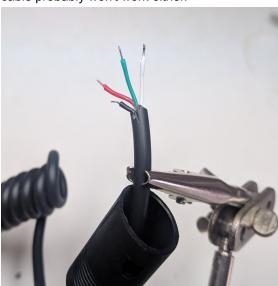
Here I have soldered a 2.2K resistor onto the pin of the DIN jack where the PTT (black) wire is going to be attached. (Note there is a problem with this picture. That resistor is actually red-red-red even though it doesn't look like it.) This will solve the problem of the TNC getting stuck in transmit. I've used a 1/4 watt resistor here because I had some on hand. a 1/8 watt resistor would also work.
