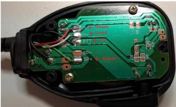
Here I've removed the 3 screws that hold the microphone back in place and opened it up. You can see that the wires are labelled on the printed circuit board, which makes it easy to figure out which wire is which. On this microphone the connections are as follows:
