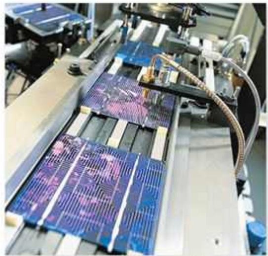
Printing of Photowatt's front-side PV cells.
