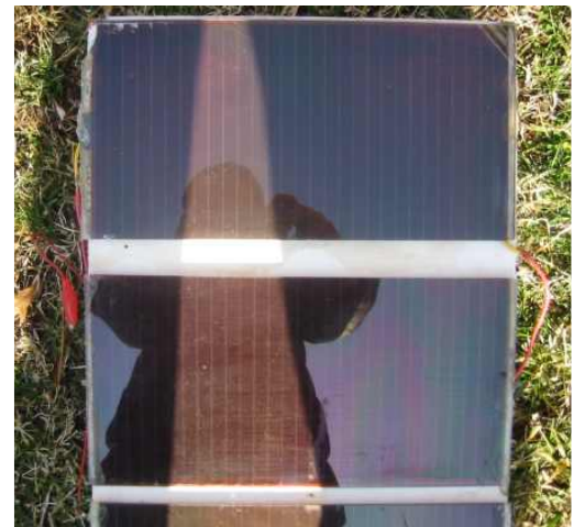
12" x 18" 12 vdc Screen Printed Solar Cells
