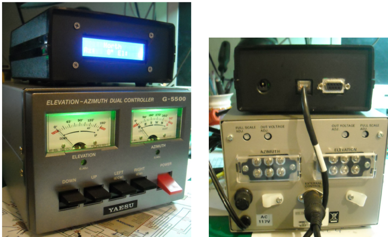
Fig. 4 – Connecting XOX TRAK Controller to YAESU G-5500 Rotor Controller
