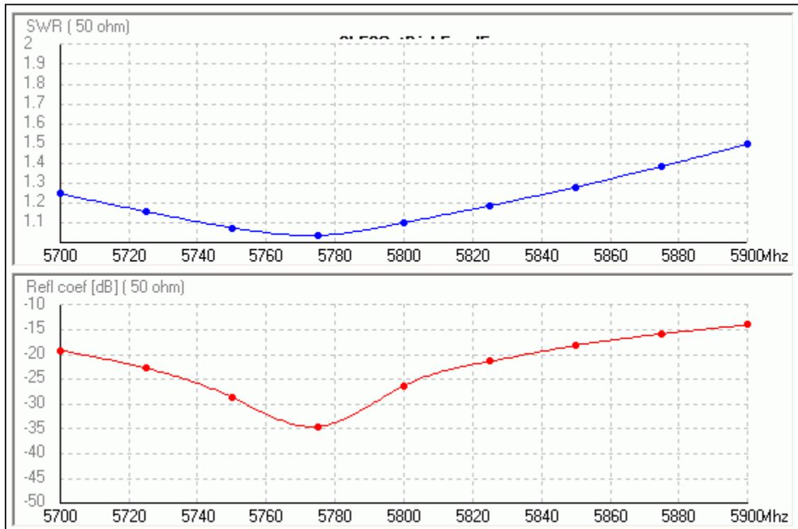
**Fig. 7. Truncated 3D Corner Reflector Feed input matching**
