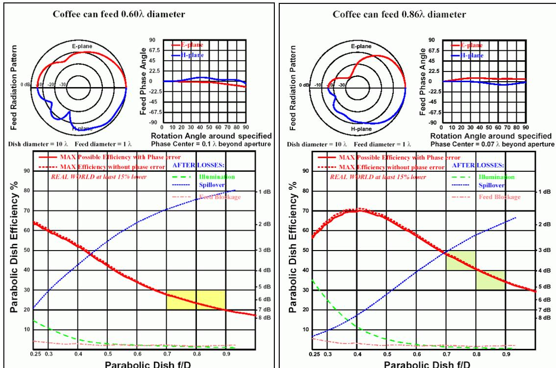
**Fig. 2. Offset parabola efficiency with 31 and 44 mm diameter coffee can feed at 5.8 GHz frequency.**
