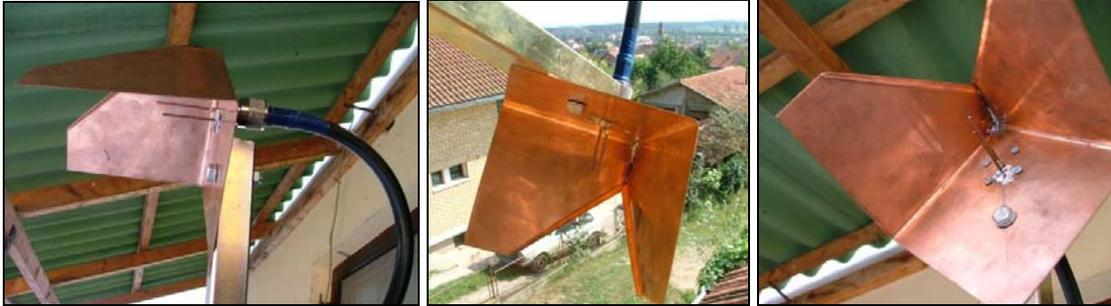
*Fig. 20. Outlook of Truncated 3D Corner Reflector Feed mounted in focus of offset parabola*
