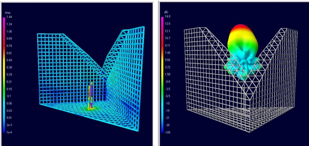
*Fig. 11. Elements current and back lobes of Truncated 3D Corner Reflector Feed*
