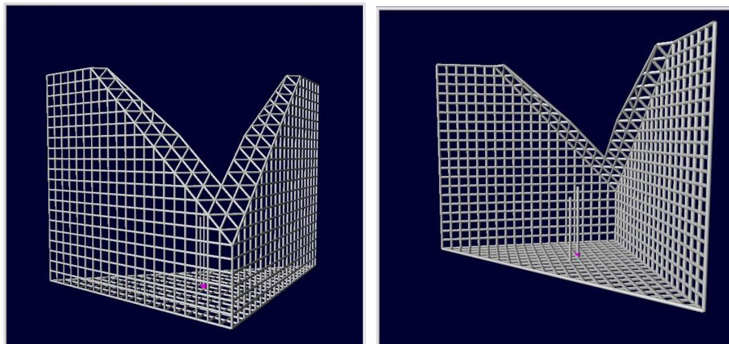
*Fig. 12. End view and side view of Truncated 3D Corner Reflector Feed*
