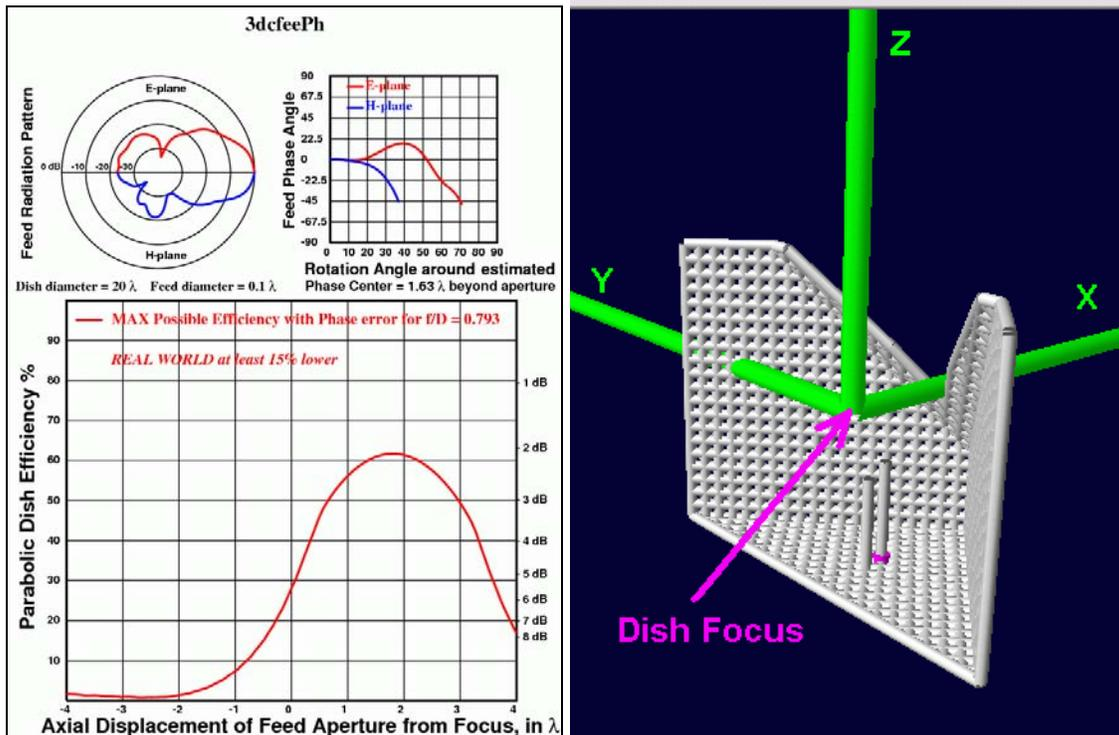
**Fig. 15. Phase center position of Truncated 3D Corner Reflector Feed and its location in relation to parabola focus**
