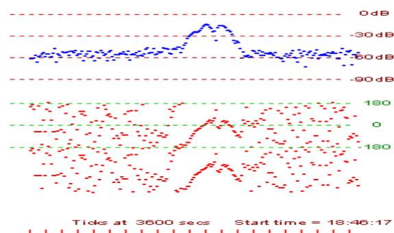
Fig. 39. A Clicklock plot of German station DCF77 (137 kHz) received in NZ
