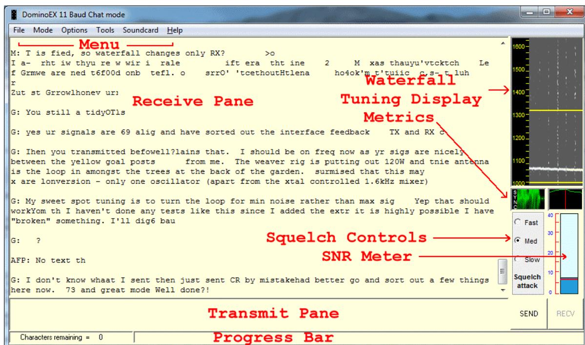
Fig. 59. The introductory screen for DominoEXChat
