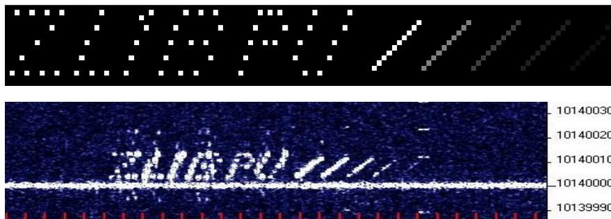
Fig. 45. Source image (above) and resulting signal (below)
