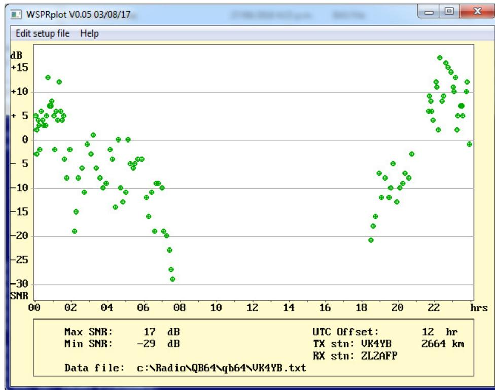
Fig. 71. WSPRplot of VK4YB running WSPR on 474 kHz, as received by ZL2AFP
