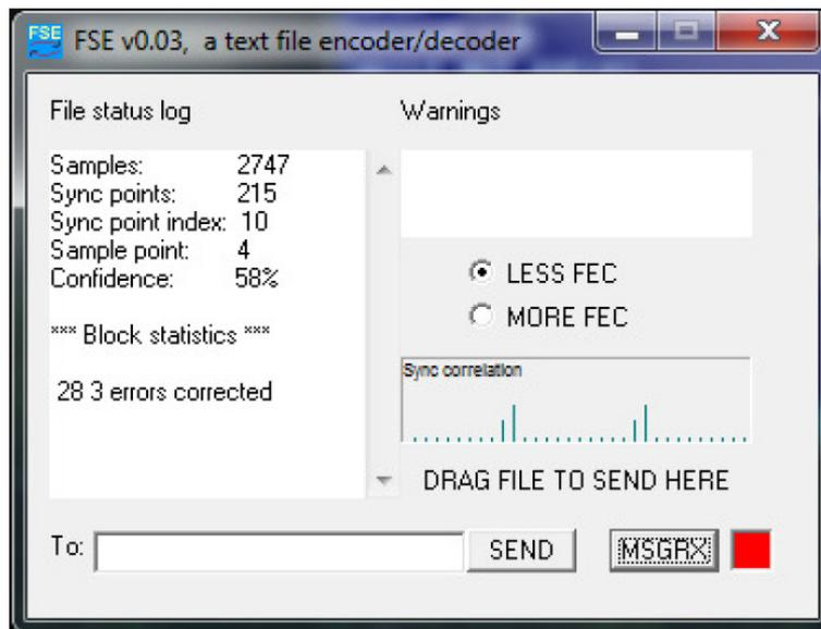
Fig. 68. The FSE error correction helper program.
