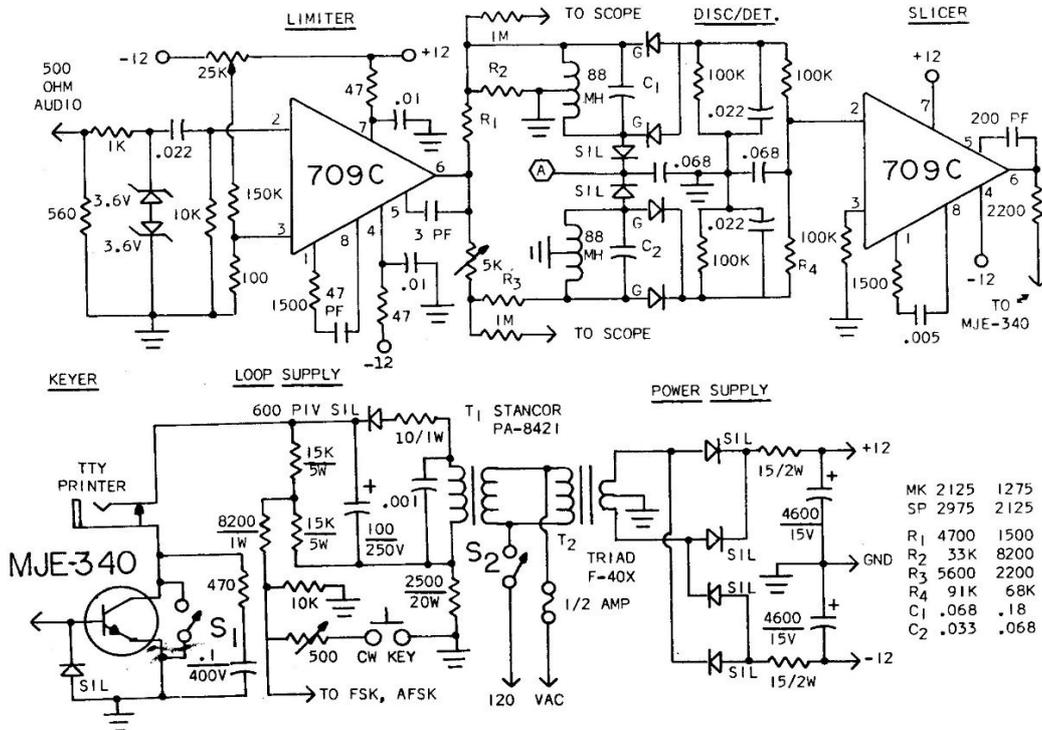
Fig. 2. The original ST-5 demodulator, RTTY Journal, May 1970
