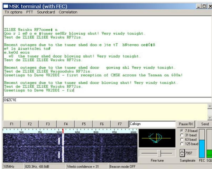
Fig. 56. VK2DDI receiving ZL1EE CMSK on 472 kHz
