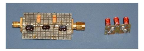
The filter should be in a shielded enclosure. It can be in the same box as the preamp. Separate modules will allow some extra versatility and if connectors are used, will allow changing filters designs easily.
