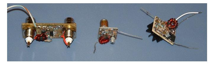
The above photo shows a few of the surface mount assemblies produced by W4EDS (SK). Ed submitted them to me for evaluation. They performed superbly. Note the size of these modules. The core diameter is 3/8 inch. Variations using 2N5109 as well as the DCP68 are shown. The wires hanging off the edges are mine and used for testing on the bench, usually input, output, Vcc, and ground.
