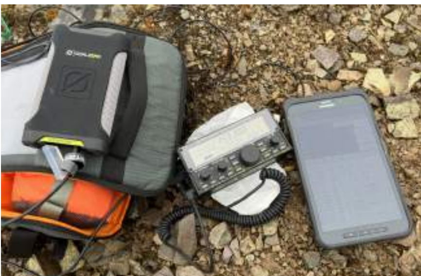
Goal Zero power pack, USB PD Cable, KX2 and VK portalog running on Samsung Tablet. Authors Image
