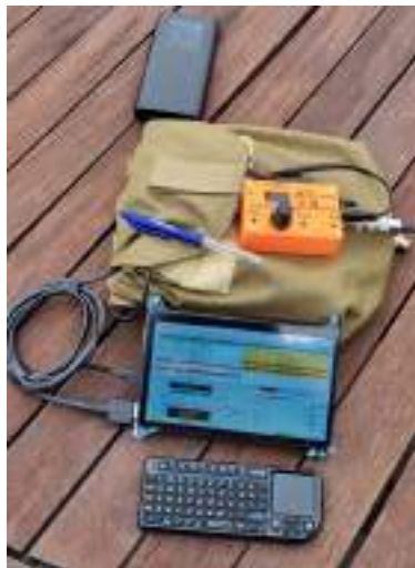
Matt ZL4HZ Digital and phone set up using the (tr)uSDX Rig - Image courtesy Matt Kerr.
